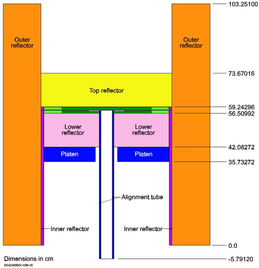
**Figure A-2:** Vertical slice through the central region of the benchmark model (not to scale).
