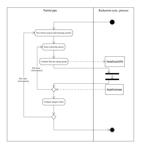
Figure 1 describes the reduction process that is used in MoC parallel solvers. The main idea is to distribute the tracks over processors. In the case of hybrid machines, each node can have more that one processor, and we speak of *ppn*: processors per node. The minimal requirements to obtain local angular flux values over each processor of a node are that:
