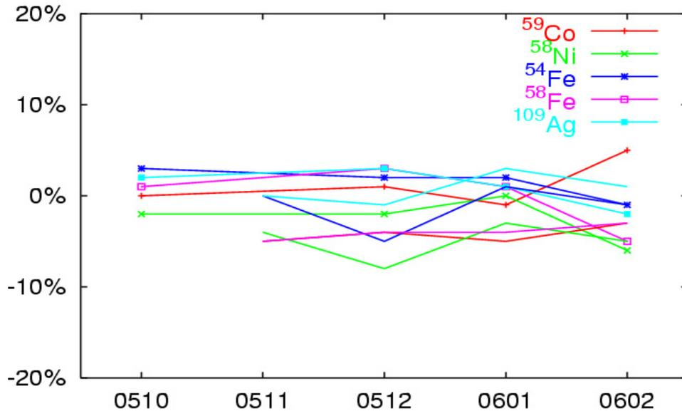
As can be seen from Fig. 6, the results of the absolute comparison of reaction rate values between calculation and measurement are well within 10% for all cases. This, in combination with the Cu wire results, justifies the use of a 10% uncertainty margin in the power values when used in the thermal hydraulics calculations. In fact, the differences between calculation and reaction rate measurements are of the order of 3% in most cases.
