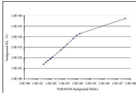
Figure4: U-238 background XS at U=4%, T=922K, W=10%
