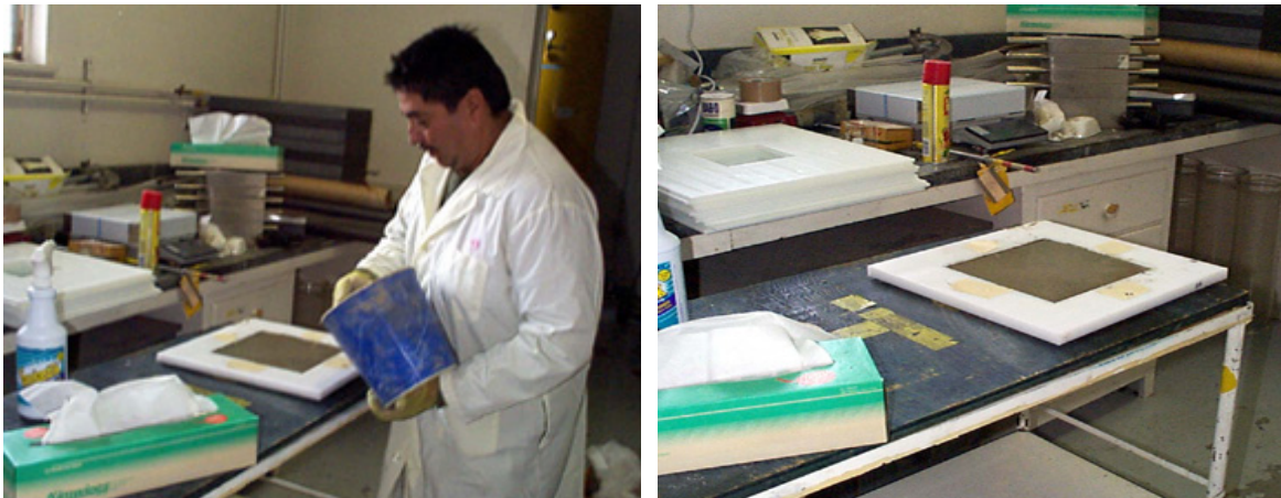
Figure 1. Concrete being poured into the recess of the polyethylene plates.
