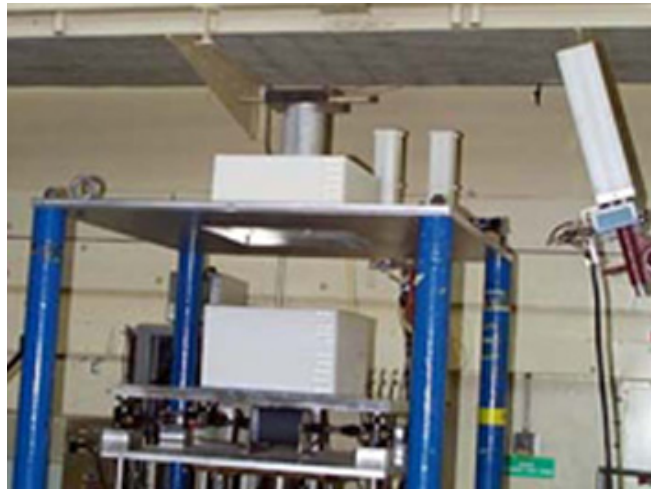
Figure 3. HEU-concrete experiment mounted on the Planet assembly.
