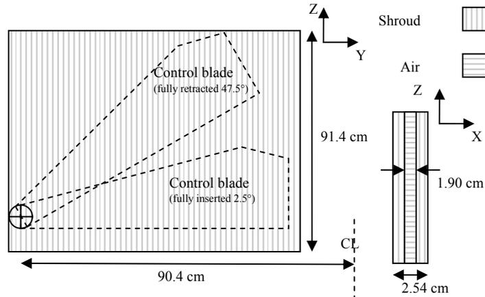
**Figure 2** UFTR Control Blade and Magnesium Shroud
