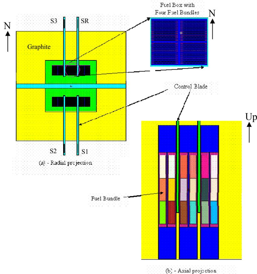
**Figure 1** UFTR Core Schematic
