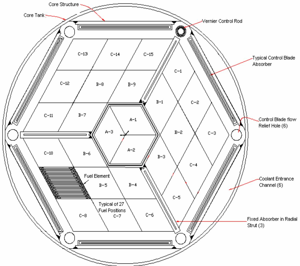
**Figure 2:** Isometric view of the MIT Reactor
