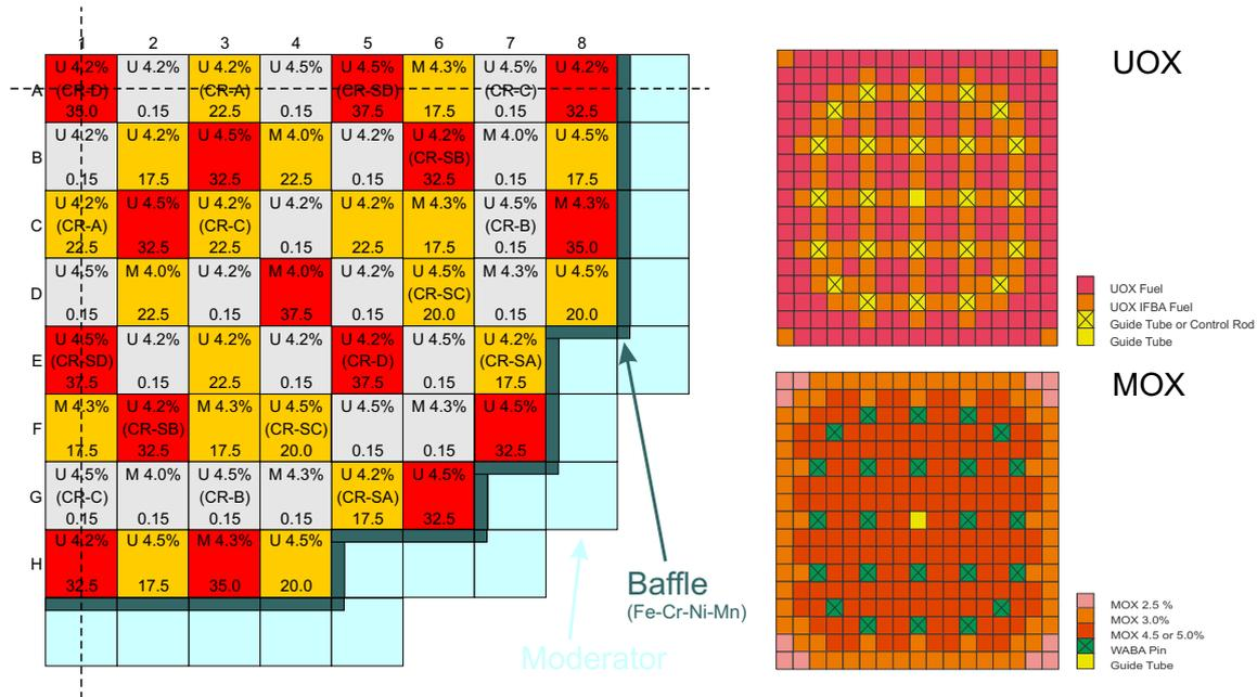
loaded with MOX fuel. In order to allow for a realistic simulation, the problem chosen for this benchmark represents a four-loop Westinghouse PWR core with a 30% MOX fuel loading.
