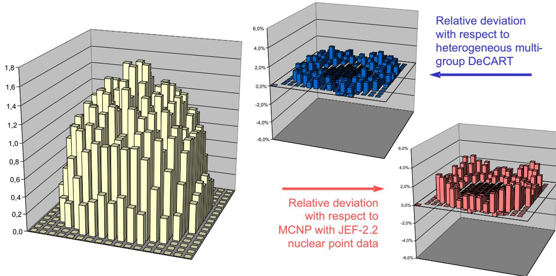
**Figure 3:** Left: Normalised pin-wise power distribution of assembly F6 of the ARO reactor state obtained from the DORT  $S_4$ - $P_1$  calculation using pin cell homogenised 16-group cross sections in  $P_1$  scattering order. Right: Relative deviations of this distribution with respect to the DeCART 47-group and our MCNP nuclear point data solution.
