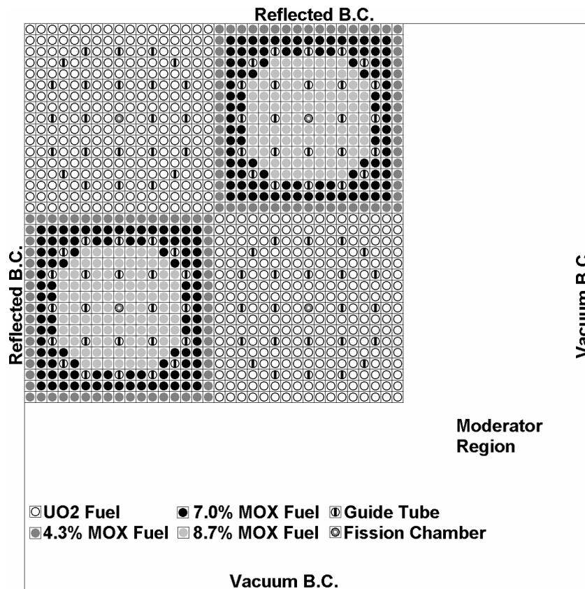
**Figure 2 OECD/NEA Two-Dimensional Benchmark configuration**
