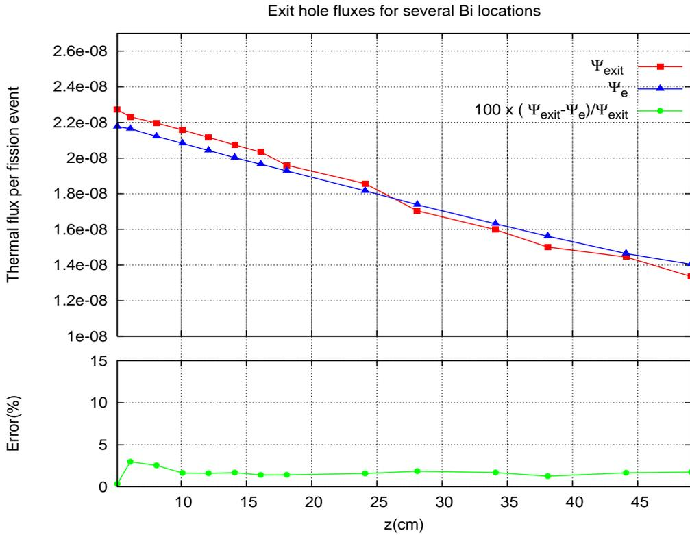
**Figure 4:** Comparison of the exit hole fluxes for the model with graphite
