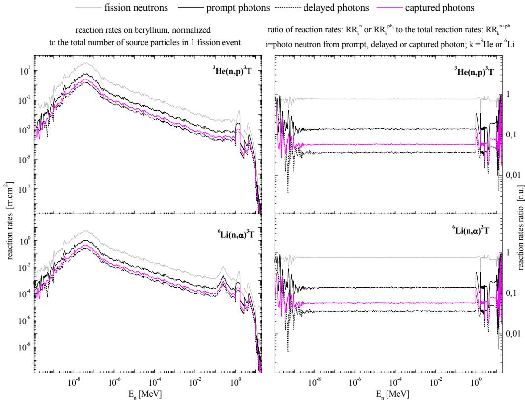
If we normalize the reaction rates by photo neutrons  $RR_k^{ph_i}$  for the nuclide  $k$  to the total number of photons of type "i", generated in fission as demonstrated at Fig. 2, then we obtain the following ratios:
