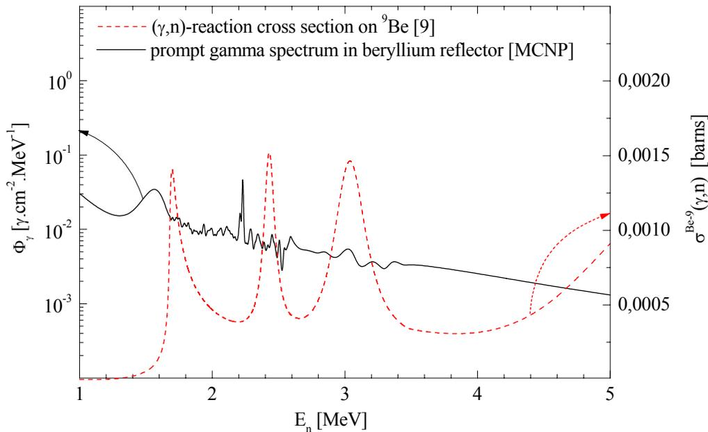
During the reactor operation a large gamma flux exists inside and around the core. The intensity of the gamma flux is about ~ 15 times higher than the intensity of the fission neutron flux. The main emitters of photo neutrons in the reactor are:
