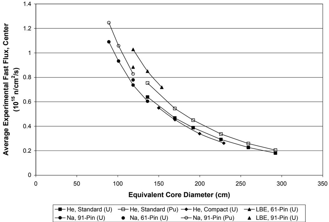
Figure 1: Average Fast Neutron Flux in the Central Experimental Position(s) as a Function of Core Diameter for Various Configuration Options.
