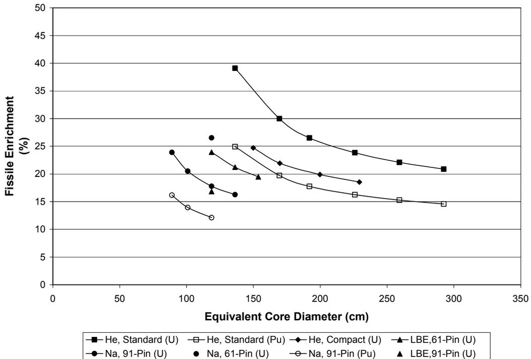
Figure 2: Fissile Enrichment Requirements as a Function of Core Diameter for Various Configuration Options.
