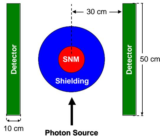
**Figure 3.** Model geometry for varying masses (radii) of shielded SNM (not to scale).
