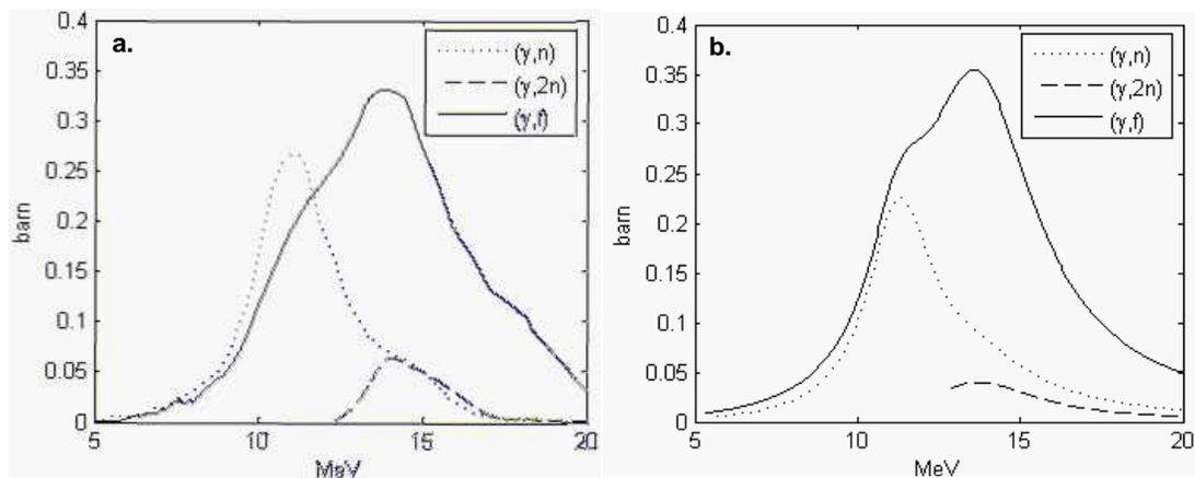
Figure 1. Photonuclear cross-sections for U-235 (a) and Pu-239 (b).
