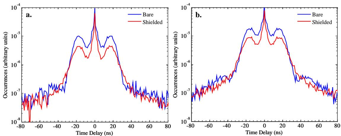
**Figure 4.** Comparison of beam-on correlation functions for spheres in bare and shielded configurations: a. 1 kg uranium sphere, b. 1 kg plutonium sphere. Shielded cases employ 20 cm of Celotex<sup>TM</sup>.
