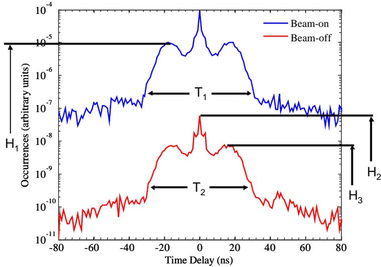
Figure 6. Sample correlation functions illustrating the features chosen as inputs for the ANN.
