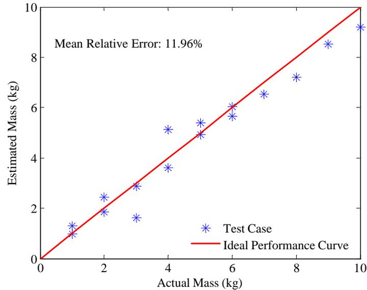
**Figure 9.** Test results for material mass using a three-layer feed-forward ANN.
