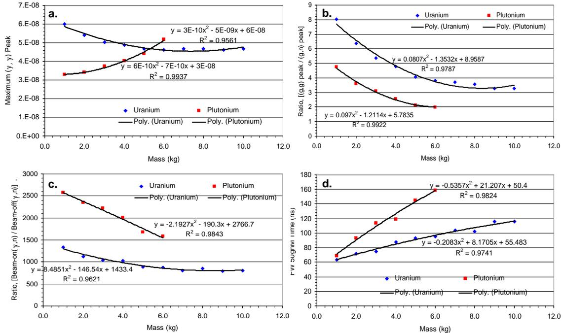
Figure 7. ANN input variables 1 – 4 plotted as a function of mass of bare uranium and plutonium spheres
