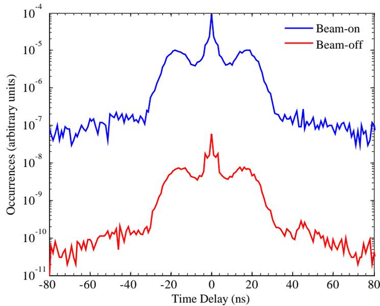
**Figure 2.** Sample detector-detector correlation function for a bare 1 kg uranium sphere.
