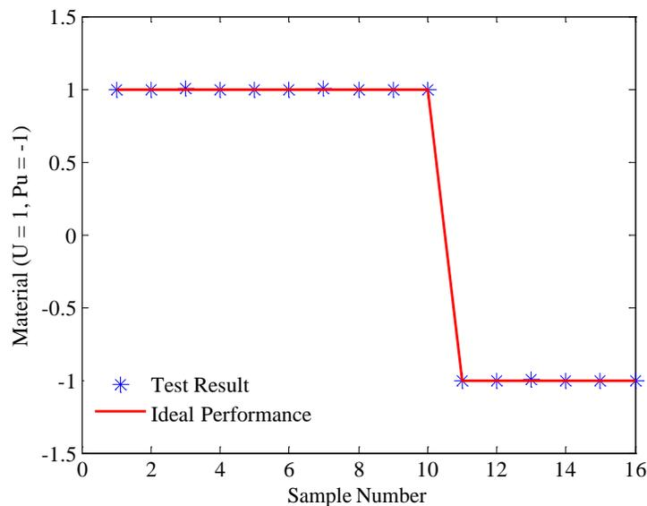
**Figure 8.** Test results for material type using a three-layer feed-forward ANN.
