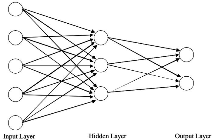
**Figure 5.** Schematic diagram of a three-layer, feed-forward artificial neural network.
