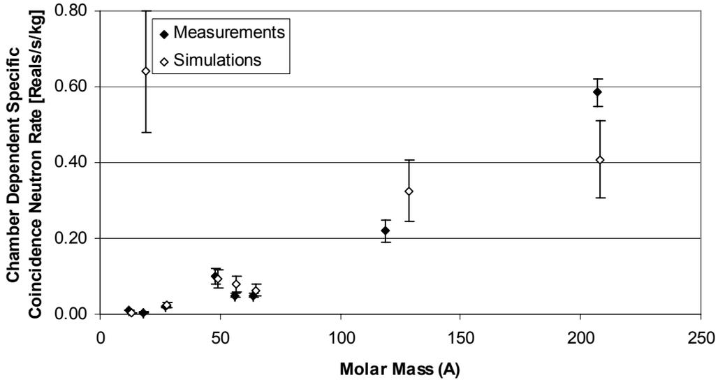
Successive simulations were run in which the counter cavity was empty, or filled with an equal volume and  $3 \text{ g.cm}^{-3}$  density of each of the materials listed in Table 1. Due to programmatic reasons, the results for Tin could not be produced at the time of this writing. Alternatively, the results for Tellurium ( $A = 127.6 \text{ g.mol}^{-1}$ ) are presented.
