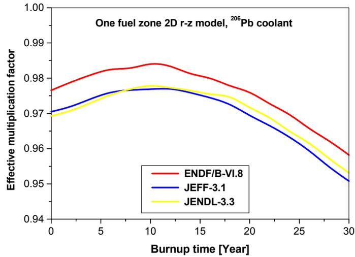
Figure 7. Comparison of  $k_{eff}$  calculations for different  $^{206}\text{Pb}$  cross-section data
