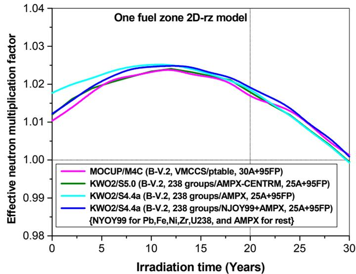
**Figure 2.** Comparison of ENDF/B-V.2 based  $k_{\text{eff}}$  calculations
