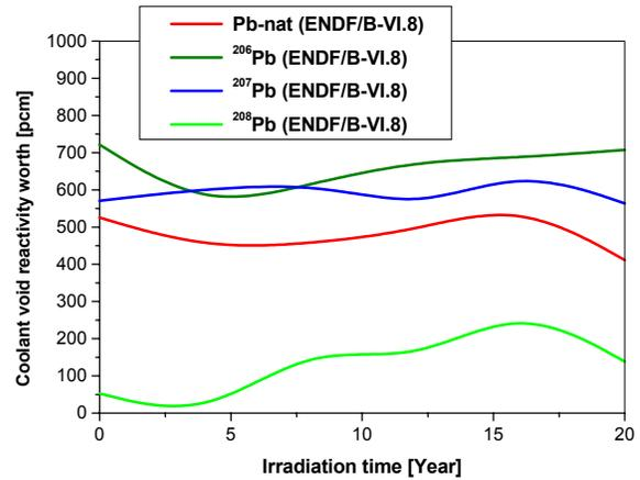
**Figure 10.** Comparison of coolant void reactivity worth for different lead isotopes
