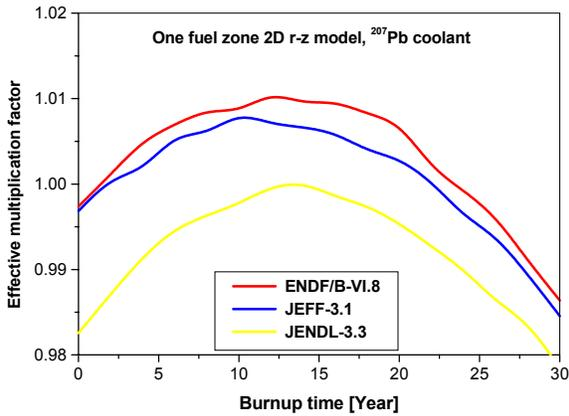
Figure 8. Comparison of  $k_{eff}$  calculations for different  $^{207}\text{Pb}$  cross section data
