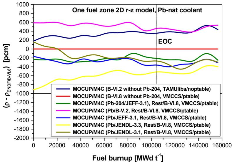
Figure 6. Comparison of reactivity calculations for different cross section data lead
