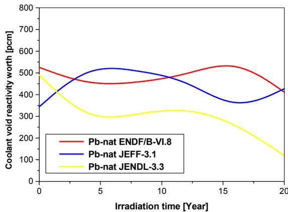
**Figure 9.** Comparison of coolant void reactivity worth for different lead cross section data
