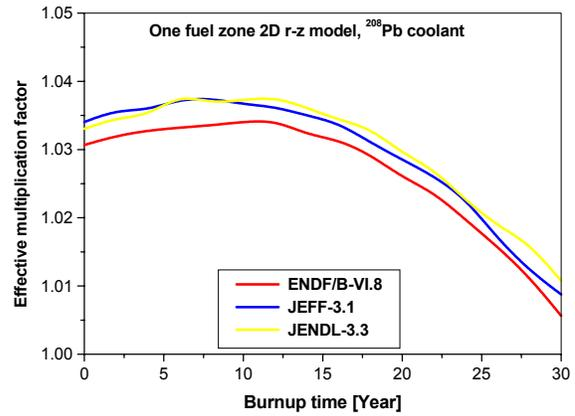
Figure 9. Comparison of  $k_{eff}$  calculations for different  $^{208}\text{Pb}$  cross section data
