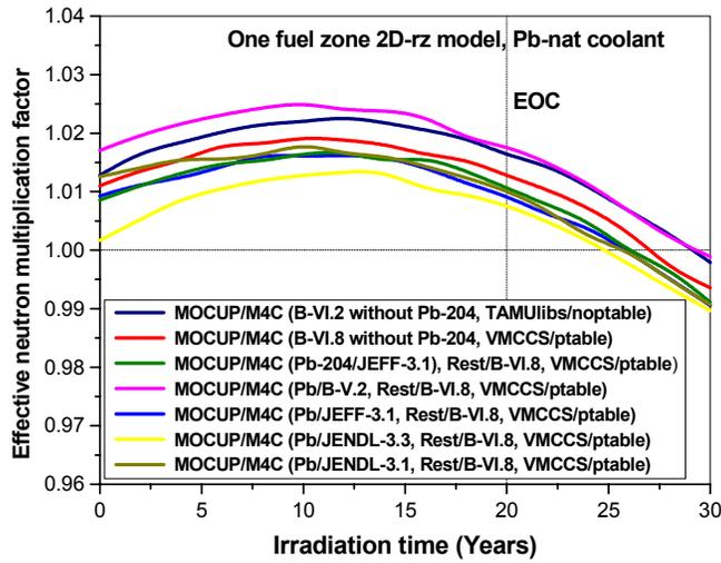
Figure 5. Comparison of  $k_{eff}$  calculations for different cross section data for lead
