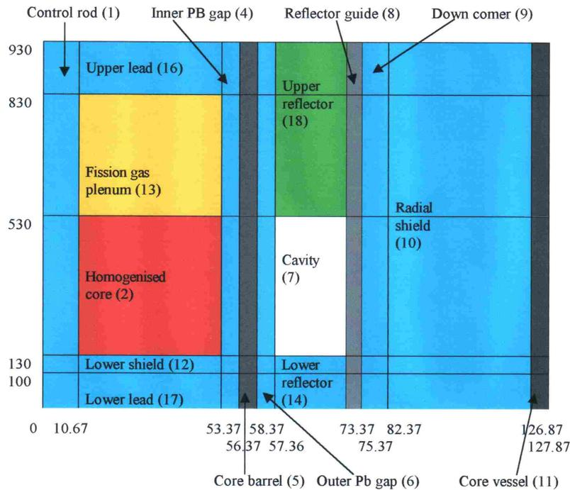
**Figure 1.** ENHS core benchmark geometry and dimensions (in cm)
