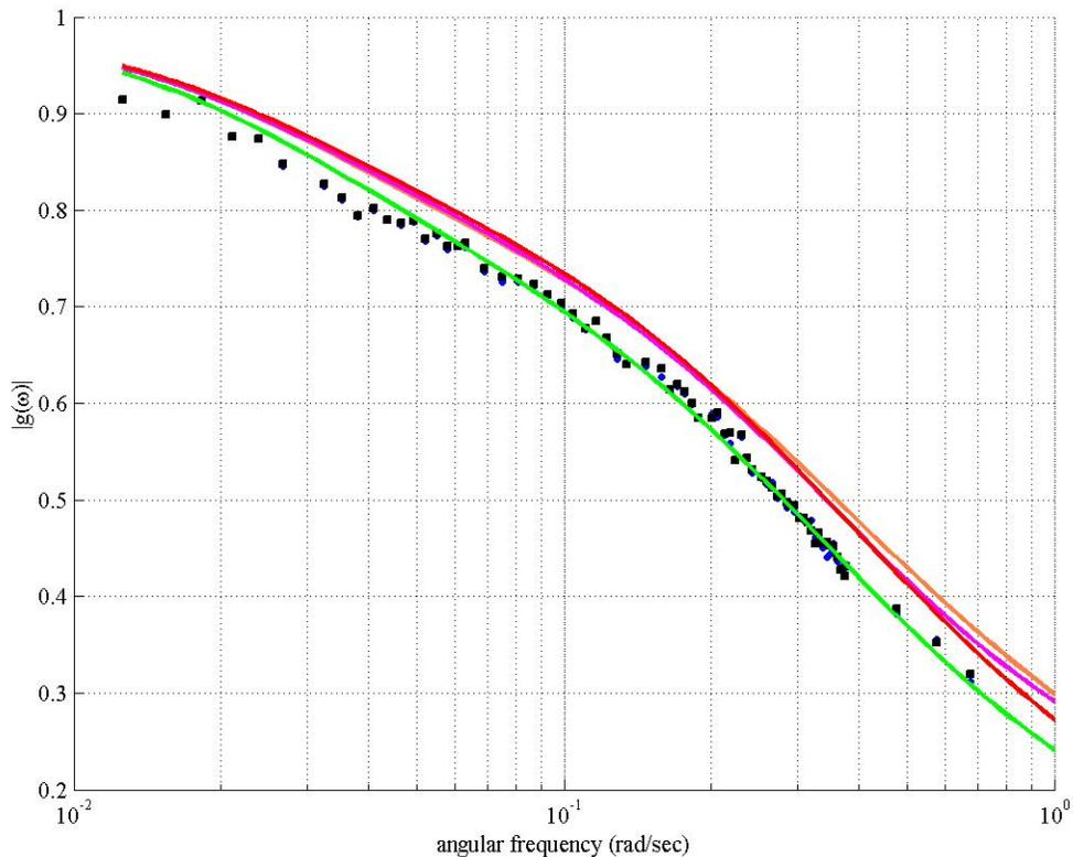
**Figure 4:** Absolute values of  $g(\omega)$ , as measured in IRR-I by the radial tunnel detector (blue) and tangential tunnel detector (black), as a function of angular frequency. Measured values are compared with calculated values based on Keepin (green), ENDF/B-VI (red), JEF-2.2 (magenta) and Brady & England (orange) group parameters.
