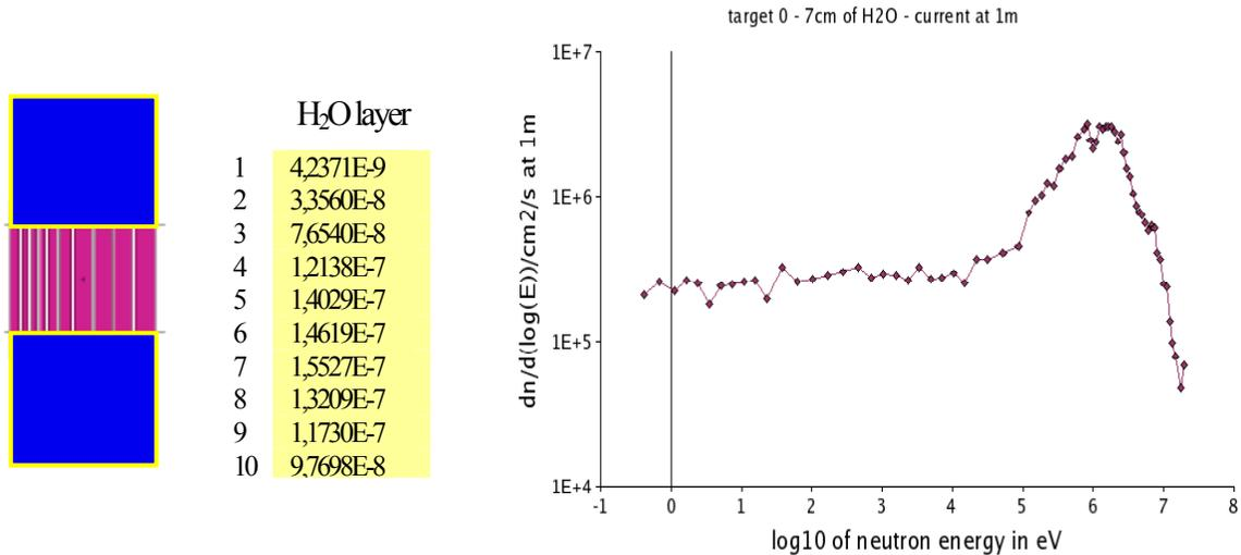
The resulting neutron spectrum is also shown in fig. 3 for 1 μA beam current. The presence of fast neutrons is unavoidable since the beam port views the target directly through the moderator, but it can be reduced by means of time-of-flight.
