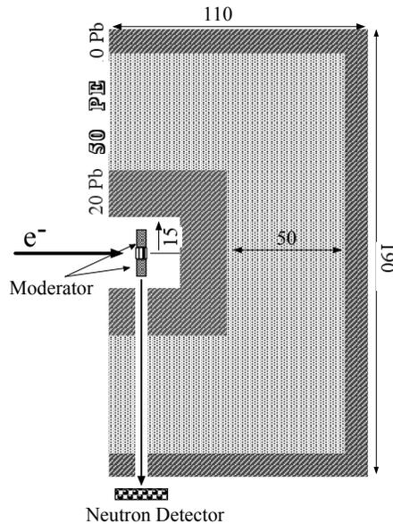
Several possibilities were investigated by means of the MCNPX code and the dose profiles on the outer surface of the dump were calculated. The simulated structure has a quadratic, rather than cylindrical symmetry, for ease of construction. No high temperature materials, like graphite, were considered, owing to the modest level of deposited power. A summary of simulated configurations is shown in Table 3.
