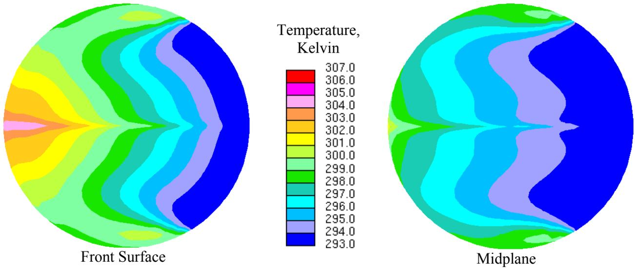
Figure 11 Front Surface and Midplane Temperature Distributions of the Coolant Channel between the Second and the Third Uranium Disks from the 100 KW Uniform Beam Using 200 MeV Electrons
