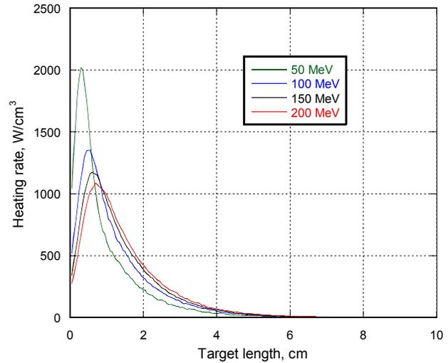
Figure 3. Spatial Energy Deposition in the Uranium Target for Different Electron Energies Normalized to 2 KW/cm<sup>2</sup> Beam Window Power Density
