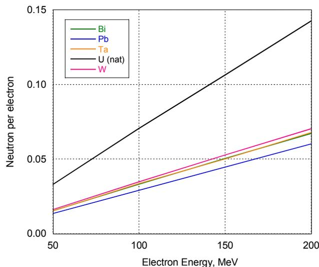
Figure 1. Neutron Yield per Electron as a Function of the Electron Energy from Different Materials
