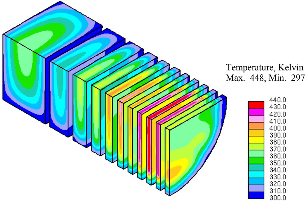
Figure 9 Temperature profiles of the Uranium Target Disks from the 100 KW Uniform Beam Using 200 MeV Electrons
