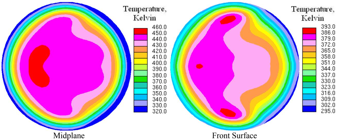
Figure 10 Midplane and Front Surface Temperature Distributions of the Third Uranium Disk from the 100 KW Uniform Beam Using 200 MeV Electrons
