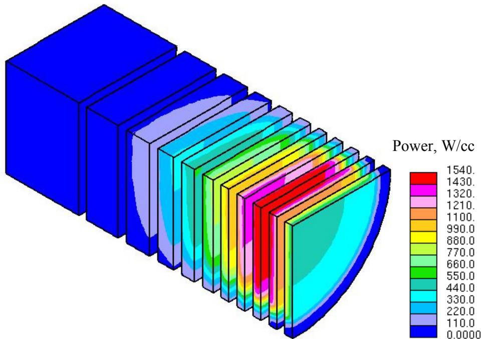
Figure 8 Energy Deposition Profiles of the Uranium Material Disks with 100 KW Uniform Beam Using 200 MeV Electrons
