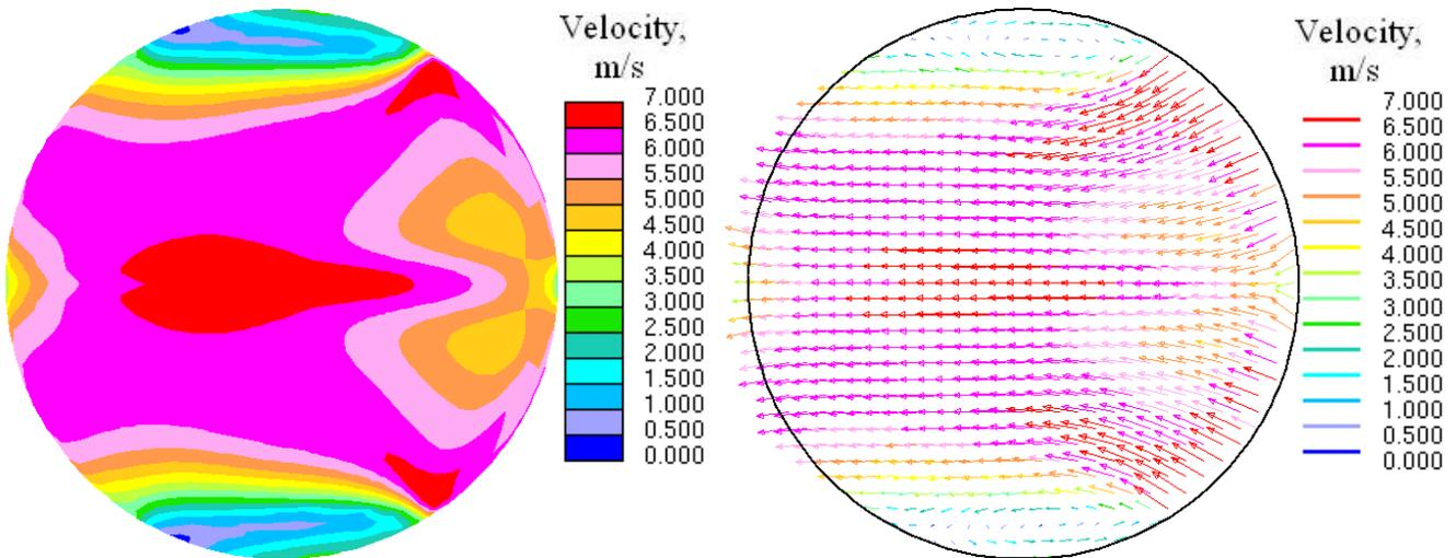
Figure 12 Midplane Flow Field of the Coolant Channel between the Second and the Third uranium Disks for the 100 KW Uniform Beam Using 200 MeV Electrons
