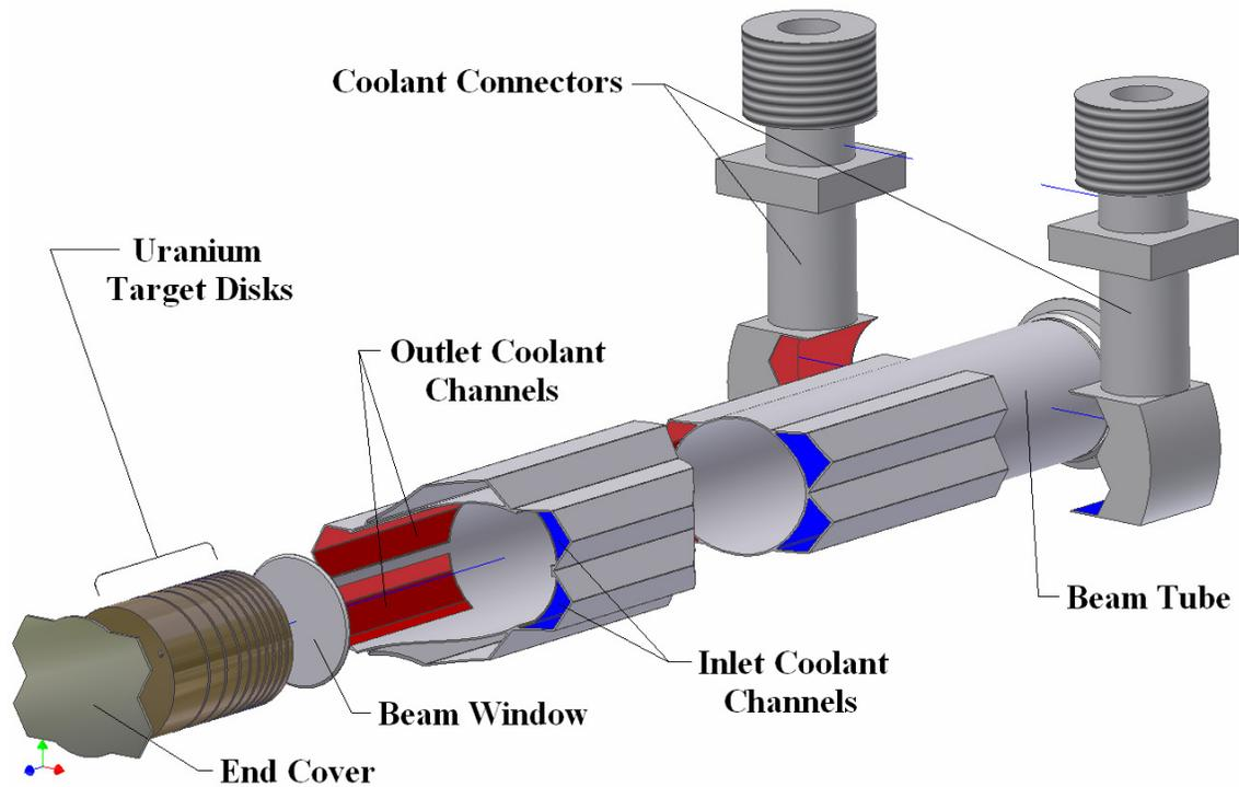
Figure 13. Exploded View of the Uranium Target Design for Hexagonal Fuel Elements
