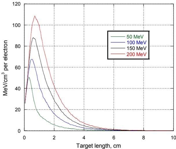
Figure 2. Spatial Energy Deposition per Electron in the Uranium Target for Different Electron Energies
