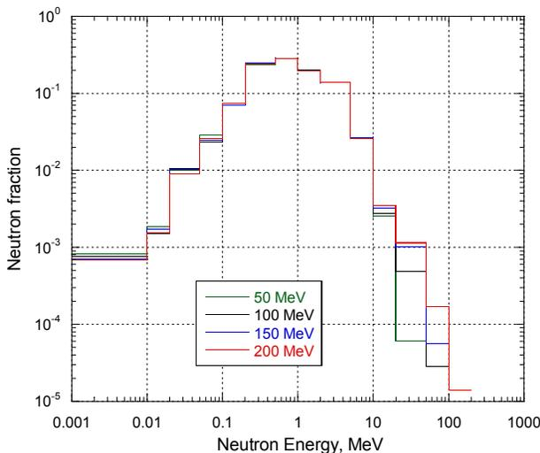
Figure 6. Normalized Neutron Spectra from Uranium Target as a Function of the Electron Energy
