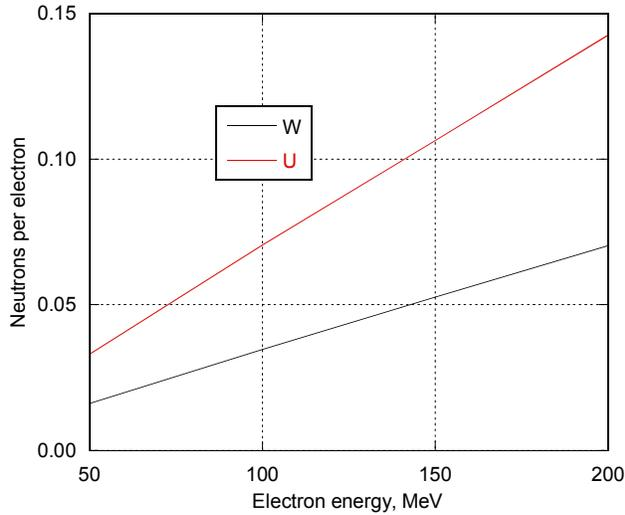
Figure 4. Neutron Yield per Electron from the Uranium and the Tungsten Targets as a Function of the Electron Energy
