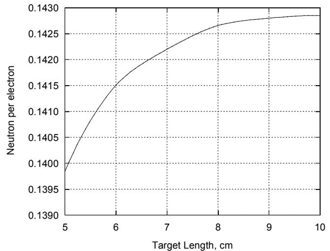
Figure 7. Neutron Yield per Electron as a Function of the Uranium Target Length
