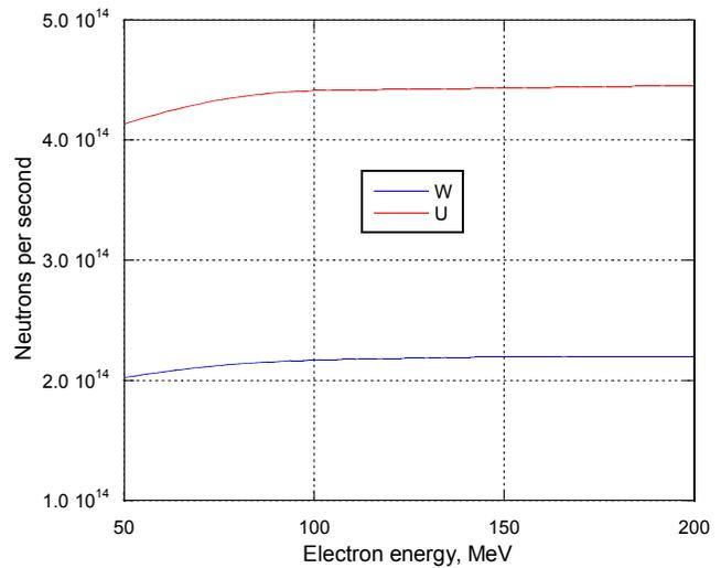
Figure 5. Neutron Source Strength from the Tungsten and the Uranium Targets as a Function of the Electron Energy with 100 kW Beam
