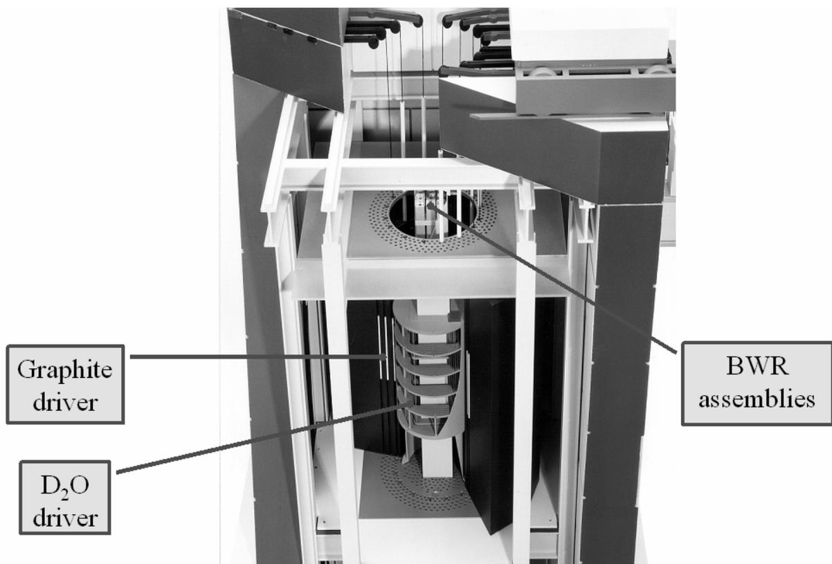
These zones are, working from the inside out; the test zone consisting of a 4.6 meter long aluminum tank containing nine BWR assemblies, the natural uranium fueled buffer zone, the 5%  $\text{UO}_2$  fueled heavy water zone, the 5%  $\text{UO}_2$  fueled graphite driver zone, and finally, the graphite reflector zone. All the control, shut-down, and safety rods are situated in the graphite driver zone,
