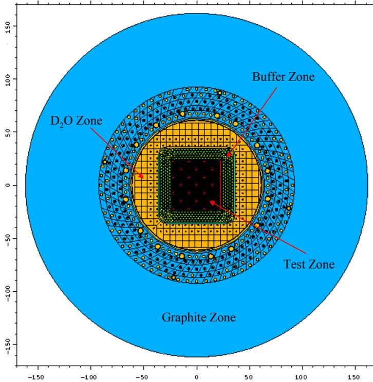
**Figure 3:** XY-cut of the LWR-PROTEUS I-1A configuration at the core mid-plane
