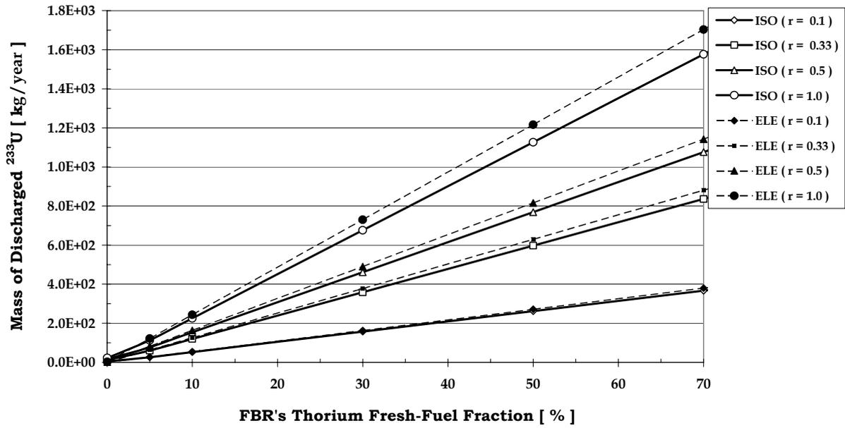
Fig. 4. Mass of discharged  $^{233}\text{U}$  from FBR in both isotopic and elemental cases
