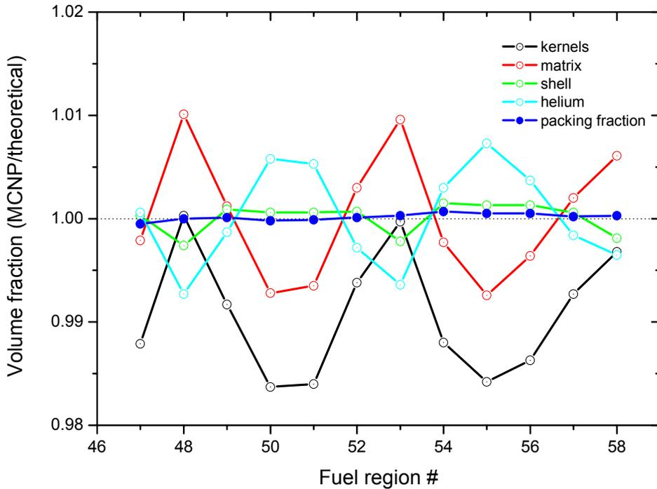
Fig. 5 allows a closer look at the fluctuations of volume fractions in channel 4. Even though the fluctuation in a kernel's volume could be as high as 2%, this fluctuation is compensated by the change in graphite volume (matrix and shell). As a result, the packing fraction and the fuel-to-moderator ratio (not plotted in Fig. 5) show a much smoother behaviour, suggesting that the overall effect on core reactivity should be limited.
