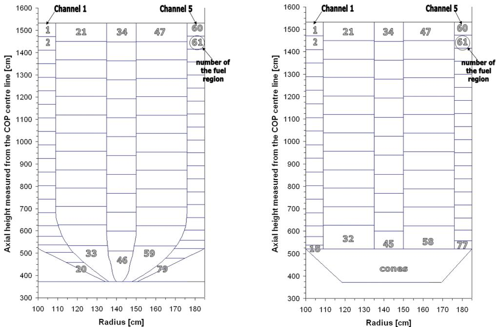
A “coarse mesh” temperature distribution derived from a fine mesh temperature distribution calculated with VSOP99, both within the core and at the graphite reflectors, was also incorporated for the first time in the model. The boundaries of this coarse mesh are determined by the available high-temperature cross-sections (XS) for graphite in the MCNP library.
