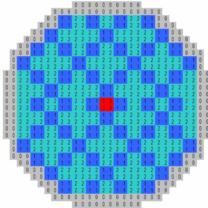
The simulations are made by a coupled 3-D kinetics/core thermal-hydraulic boundary conditions model. The developed TRACE and TRAC-BF1 model was built based on different thermal-hydraulic components. The core is modeled by 14 channels, bottom and top boundary conditions are specified in this model using the FILL and BREAK components, Fig. 2. The 14 thermal-hydraulic channels are coupled to the neutronic model according to the radial distribution shown in Fig. 3.
