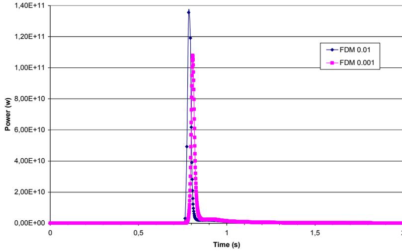
**Figure 7:** Reactor power evolution with TRACE/PARCS HYBRID and different time steps.
