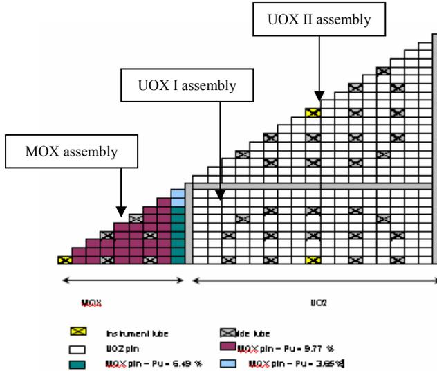
**Figure 5:** Pin power decrease on UO<sub>2</sub> assembly at the MOX/ UO<sub>2</sub> boundary
