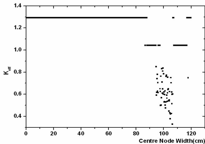
When the center node size increases to greater than about 80cm, the solution becomes unstable
