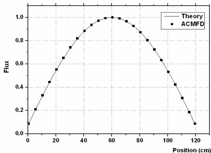
Tab. 3 shows how the iteration solution converges to the first harmonic mode for the case of 90cm center node. The nodes interior fine mesh flux reconstructed via the ACMFD coarse mesh nodal solution reproduces the analytical solution for the first harmonic mode, which is shown in Fig. 3. As one can see in Tab. 3, throughout the iteration the average fluxes in the three nodes remain positive without any direct information indicating the appearance of negative flux
