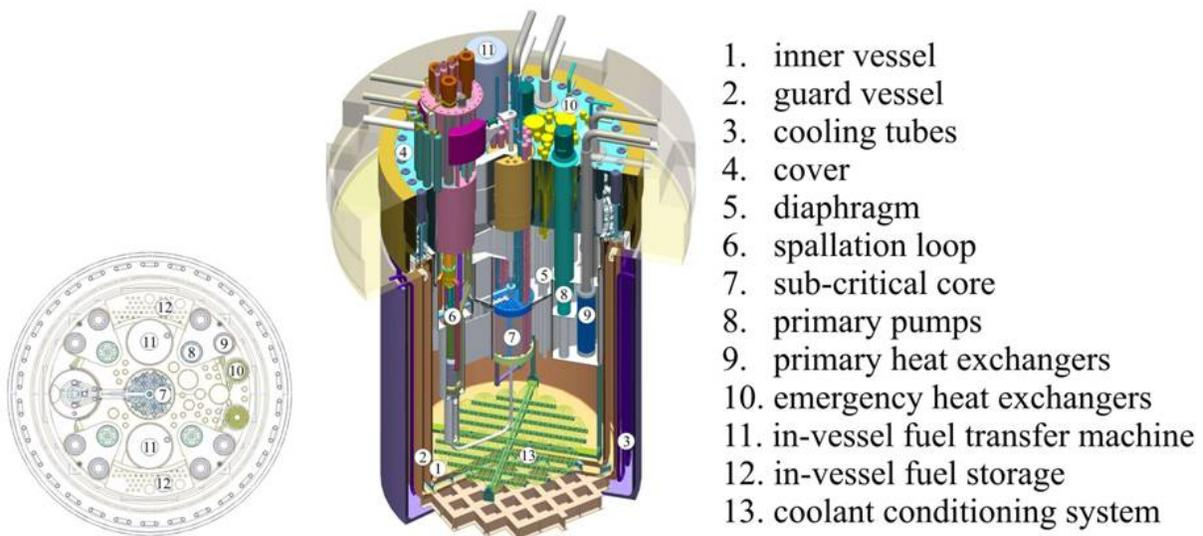
**Figure 1: bulk cut-views of the MYRRHA ADS**
