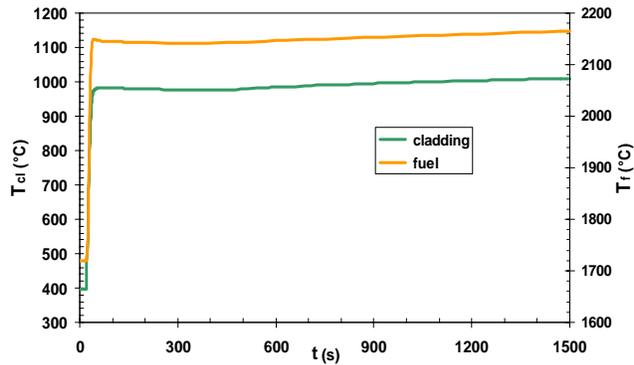
Figure 6: unprotected LOF maximum clad and fuel temperatures
