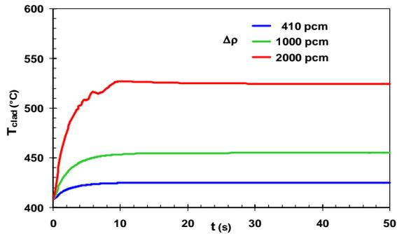
Figure 8: unprotected TOP maximum clad temperature
