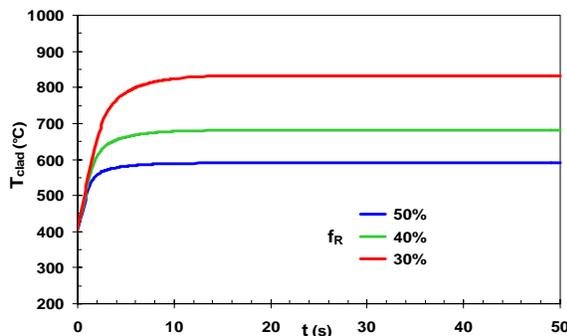
Figure 10: unprotected SA blockage maximum clad temperature
