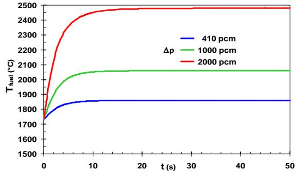
Figure 9: unprotected TOP maximum fuel temperature
