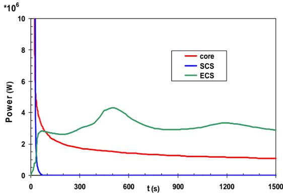
Figure 3: protected LOF&LOH core and cooling systems powers
