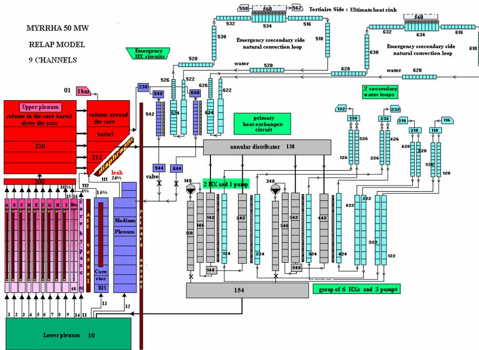
Figure 2: schematic representation of the RELAP model of MYRRHA
