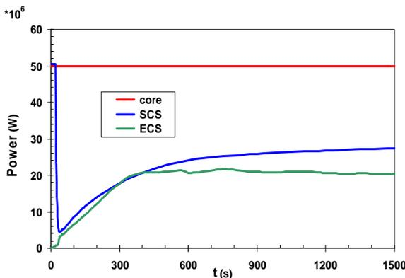
Figure 5: unprotected LOF core and cooling systems powers
