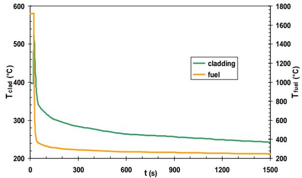
Figure 4: protected LOF&LOH maximum clad and fuel temperatures
