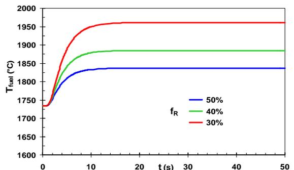
Figure 11: unprotected SA blockage maximum fuel temperature
