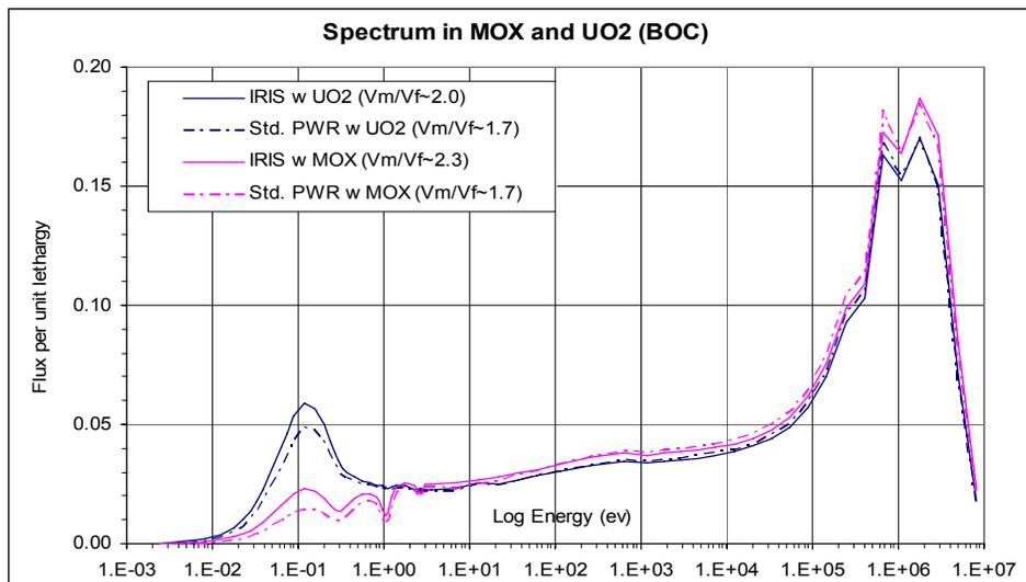
**Figure 3:** Spectrum in UO<sub>2</sub> and MOX with IRIS and standard PWR lattice (40 GWd/tHM)
