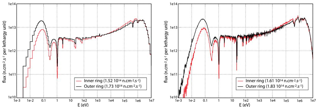
In terms of burnup, this spatial spectrum effect leads to much bigger differences on Pu-239 depletion between Th/Pu fuel rings than on U-235 depletion between  $U_{nat}$  fuel rings. Over a bundle cycle, the Pu-239 mass variation within the inner (outer) fuel ring of the Th/Pu bundle amounts to 0.58 (1.29) times the average mass variation in fuel, while the corresponding ratio for U-235 mass variation in the  $U_{nat}$  bundle amounts only to 0.84 (1.10).
