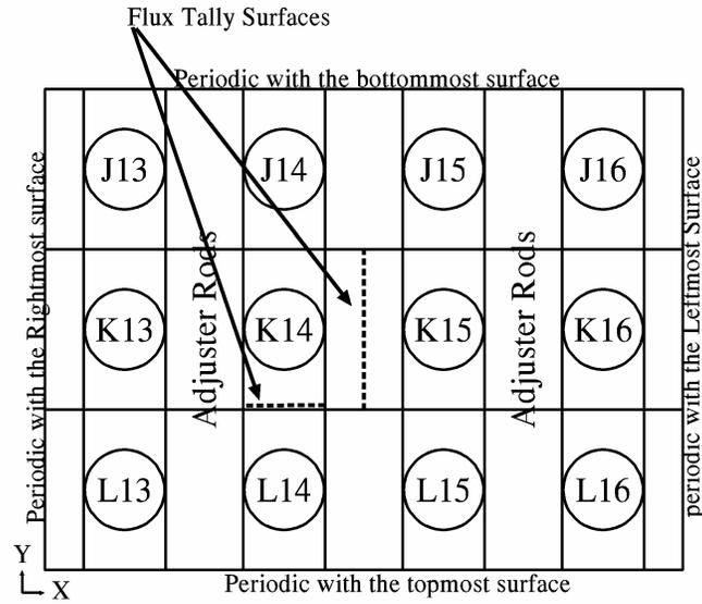
**Figure 2: MCNP sagged model: Cross sectional view in the X-Y plane**
