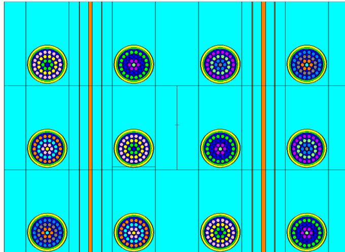
**Figure 3: MCNP sagged model: Cross sectional view in the Z-Y plane**
