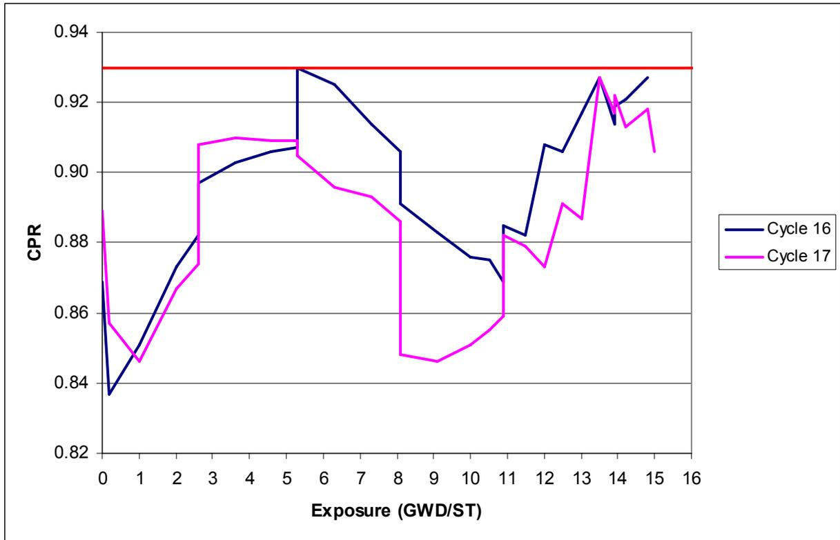
**Figure 5.** Comparison of the Maximum Fraction of Limiting Power Density (MFLPD)
