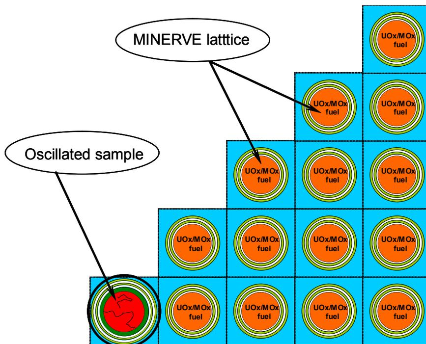
APOLLO2 calculation uses P<sub>ij</sub>-UP1 model (interface current method with linear anisotropic angular fluxes). The space-dependent (4 concentric rings in every fuel pin description) self-shielding calculation for resonant isotopes is performed using the Probability Table method. Modeling errors were assessed [6] by comparison with the reference continuous-energy Monte-Carlo calculation TRIPOLI4 [7].
