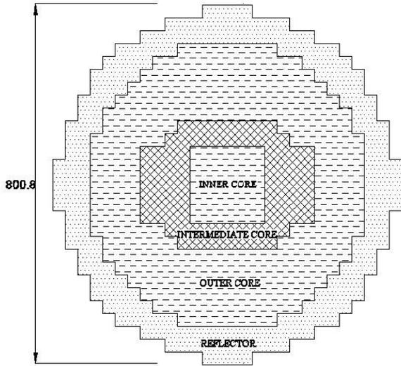
**Figure1(b):** Details of power zones in PHWR
