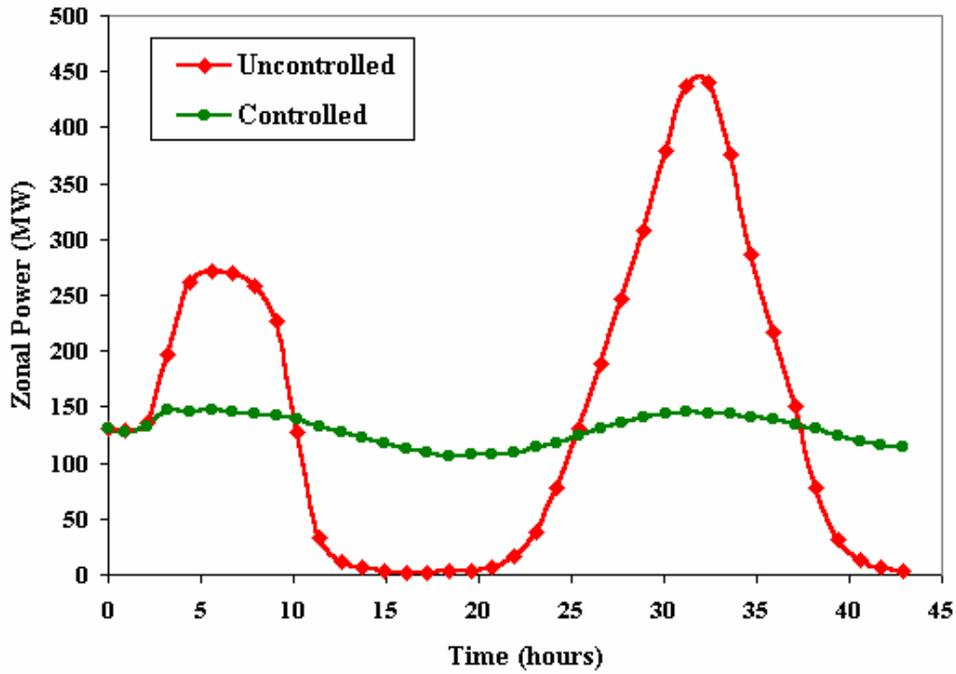
**Figure 6:** Tilt based Control scheme (Power variation in zone 1)
