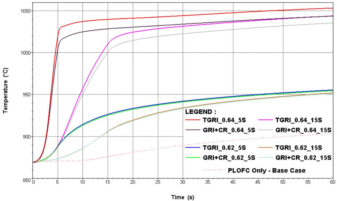
**Figure 6:** Maximum fuel sphere centre temperature envelopes for an SSE event followed by PLOFC or DLOFC conditions
