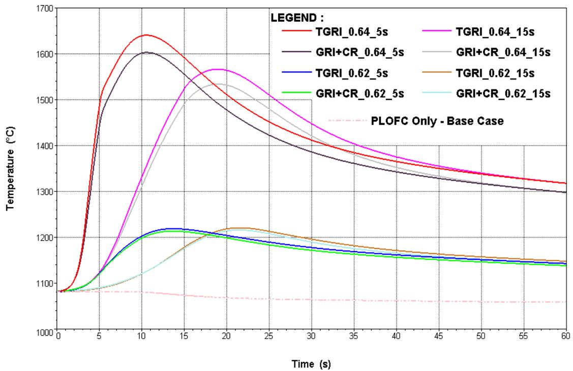
**Figure 5:** Core average fuel sphere temperatures for an SSE event and PLOFC conditions
