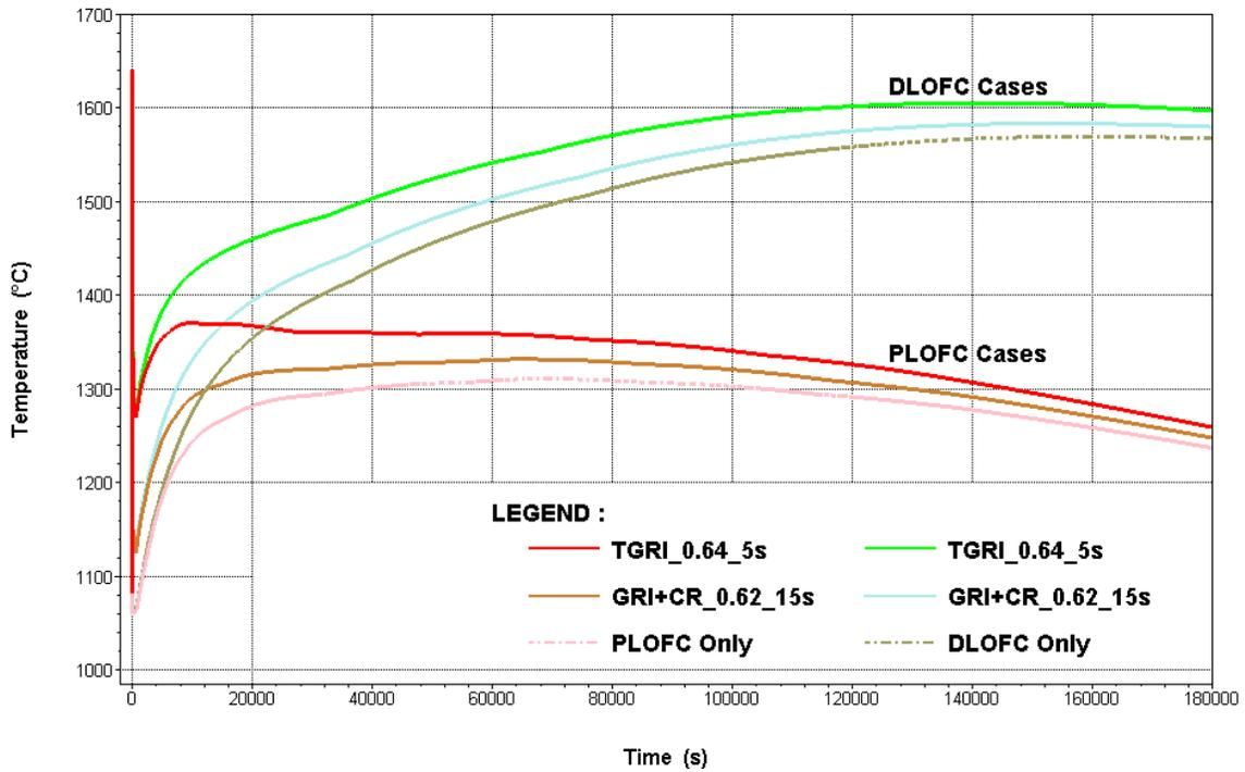
**Figure 7:** Core average fuel sphere temperature envelopes for an SSE event followed by PLOFC or DLOFC conditions
