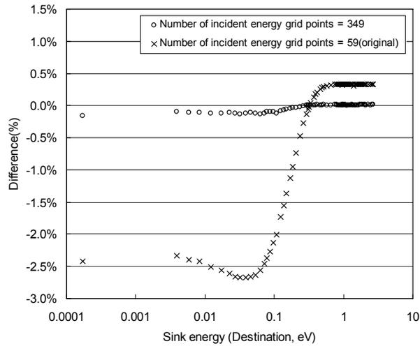
Comparison of neutron spectrum between AEGIS using the modified AELIB and MCNPX are shown in Fig.5. From Fig.5, discrepancy between the two codes are reduced and both codes show good agreement.
