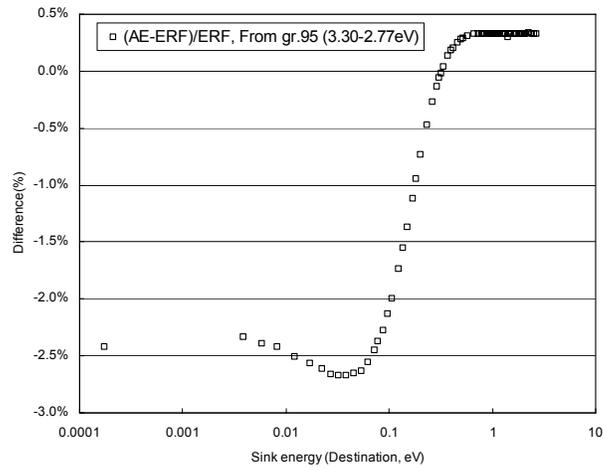
**Figure 4:** Difference of scattering matrix of H (from group 95, 3.30-2.77eV) between AELIB and analytical value obtained by the error function (ERF)
