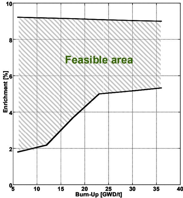
**Figure 7** Required uranium enrichment on feasible area of breeding for cell 2
