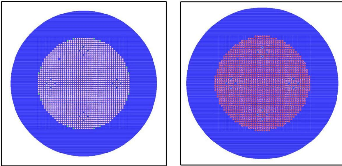
**Figure 1:** MISTRAL2 and MISTRAL3 radial cross sections
