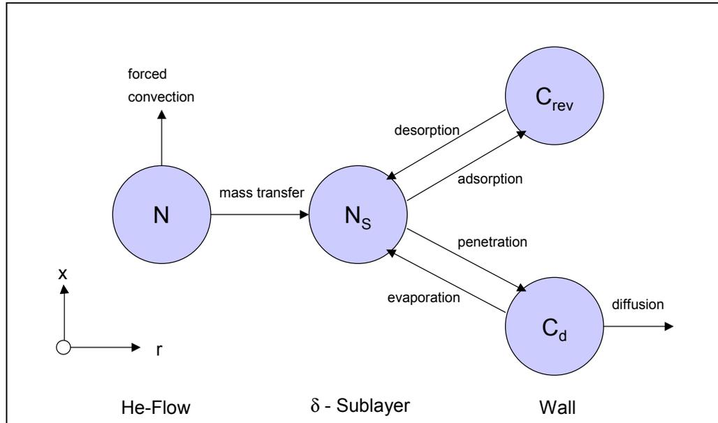
The transport rates between above reservoirs are based on the following physical processes:
