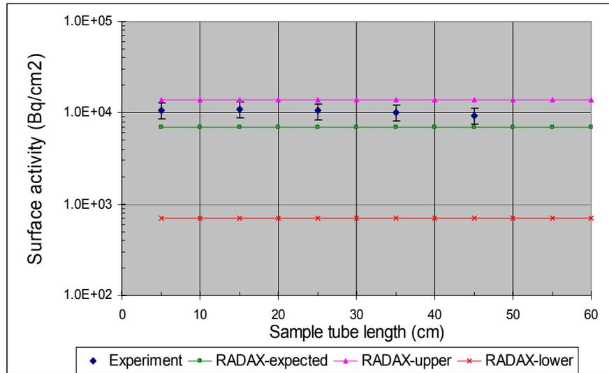
The results of the comparison between RADAX calculated and experimental results at the end of the respective LAMINAR-loop runs, (one example in Fig. 4), show very good correlation.
