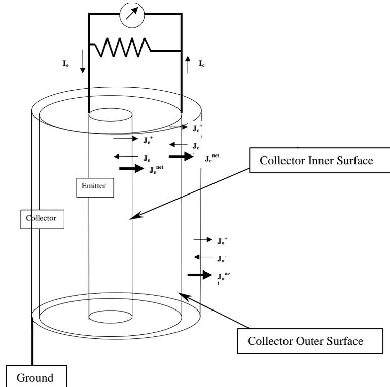
Figure 2 Schematic of the Electron Flow in the In-core Detector
