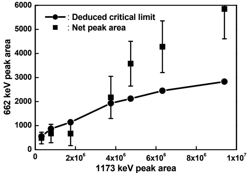
Therefore, from the above work, it is confirmed that the 662 keV peak shown in Fig. 2 is originated from a large amount of 1173 keV gamma-rays from Co-60, i.e., no doubtful nuclide about leakage of reactor pool water is found in the water collected from the beam tube of HANARO.
