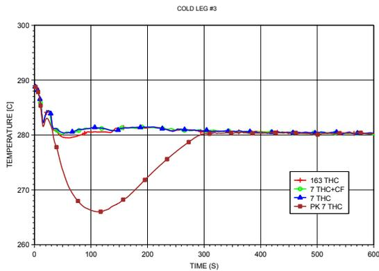
**Fig. 6** Comparison of cold leg #4 coolant temperature in case of 163 THC, 7THC with and without CF and point kinetics
