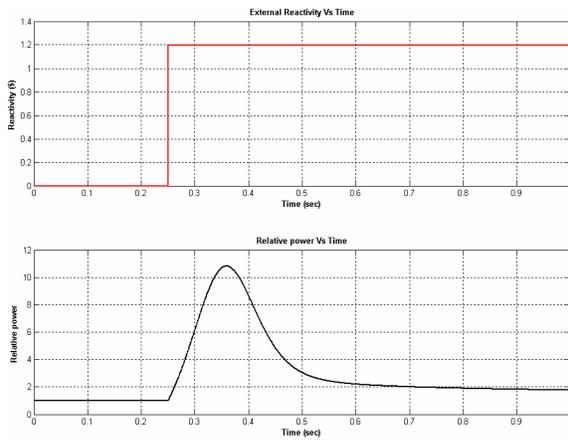
**Figure 3: Ramp transient**
