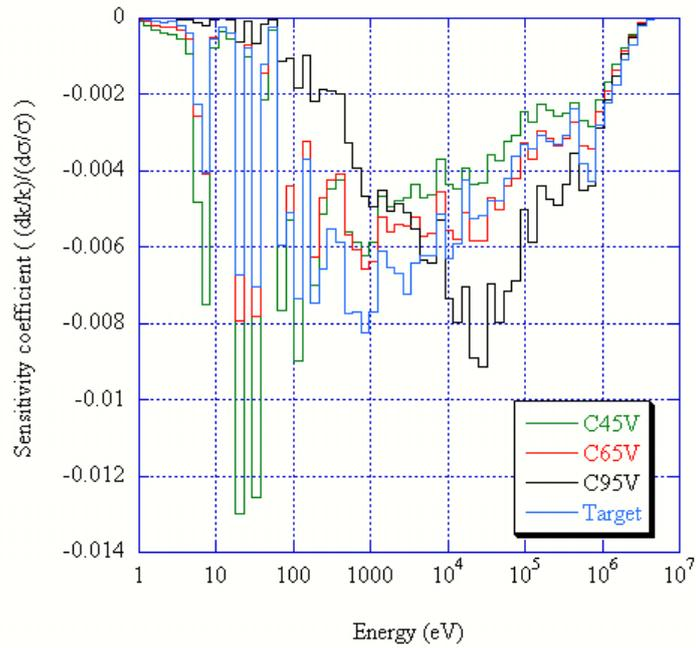
**Figure 2:** Sensitivity coefficients for  $k_{eff}$  in each core with respect to  $^{238}\text{U}$  capture cross section
