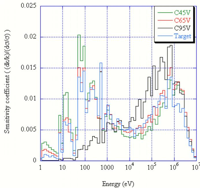
**Figure 3:** Sensitivity coefficients for  $k_{eff}$  in each core with respect to  $^{239}\text{Pu}$  fission cross section
