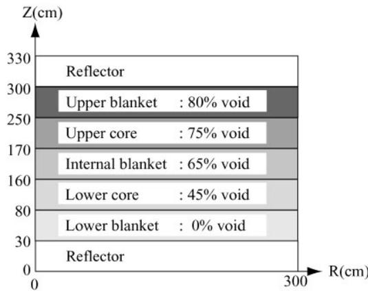
Figure 1: Calculational geometry of a target core
