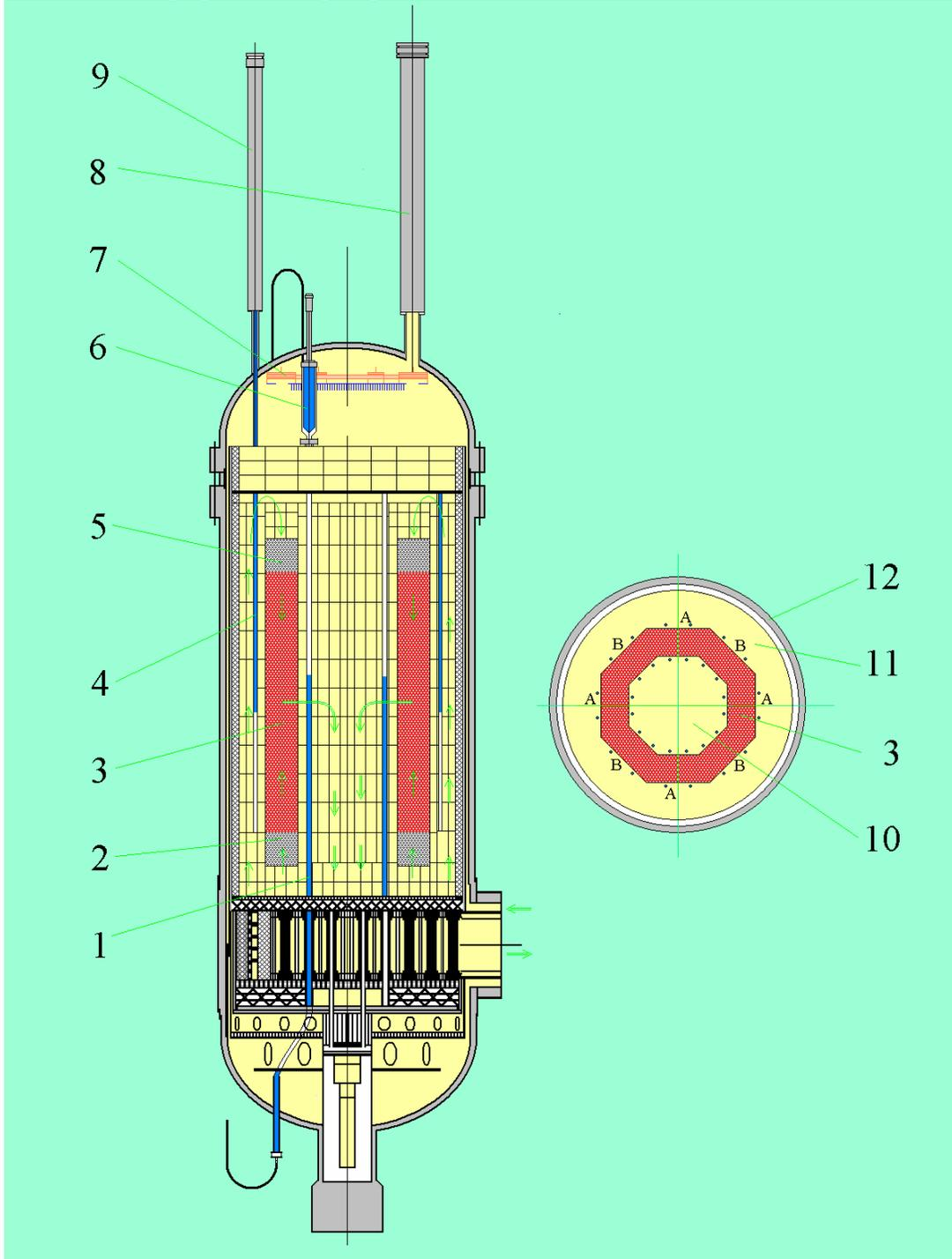
**Fig.5:** Vertical and horizontal cross-section of OBMR
