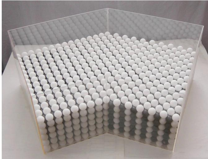
**Fig.4:** One eighth simulator of octagonal core
