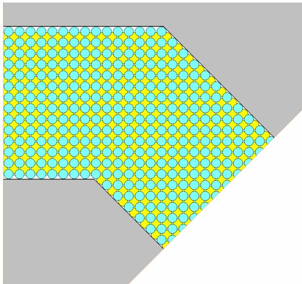
**Fig.3:** One eighth of octagonal annular core
