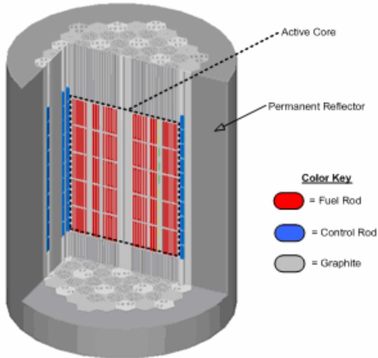
The pebble-bed core is based on China's operating High Temperature Test Module (HTR-10). The pebble bed core consists of a fuel region (active core) that has a diameter of 180 cm and a height of 197 cm. The fuel region is surrounded by graphite reflectors, which consist of top, bottom, and side reflectors. A vertical cross-sectional view of the modeled structure is shown in Fig. 3.
