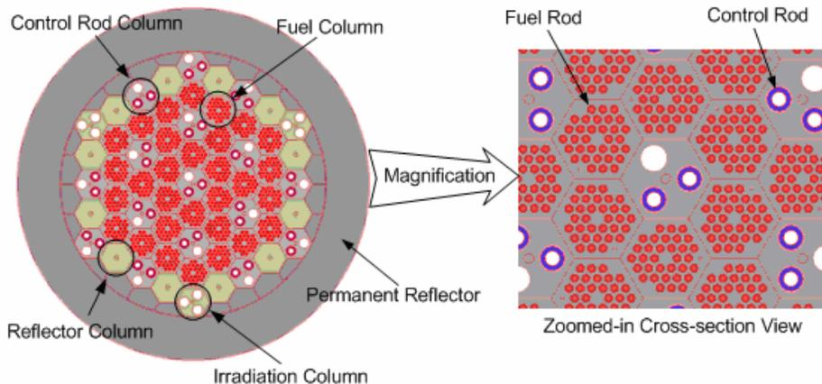
The general procedure for creating the model was to build the four types of prismatic hexagonal blocks that compose the HTTR, then to arrange these blocks in an array of rows and columns to construct the core. The completed computational model has over 8,500 lines. There are 7,290 geometry regions in the model.
