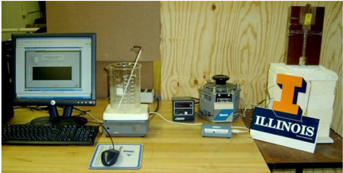
Figure 2: Boiling heat transfer experiment set-up
