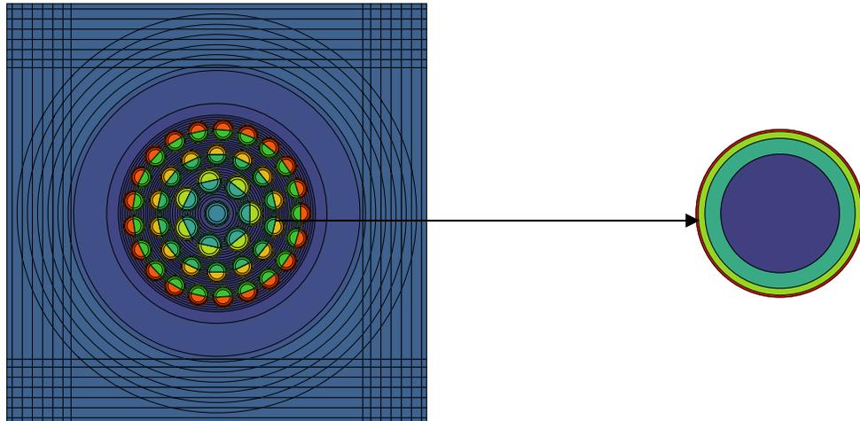
**Fig. 1: Cross section of CANDU-NG unit cell and single pin**
