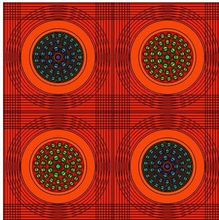
**Fig. 2: Cross section of 2x2 CANDU-NG assembly**
