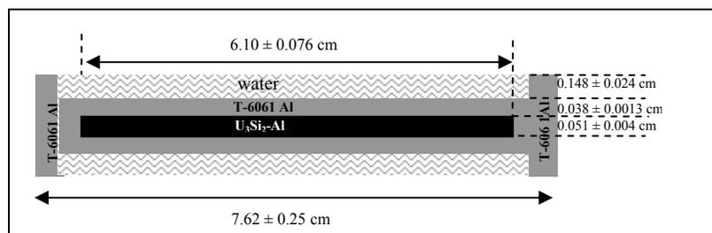
Figure 1: Schematic of the Exact Fuel Plate Geometry
