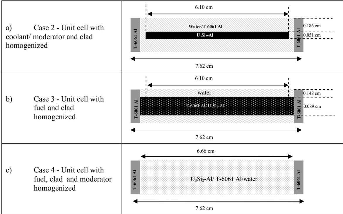
Figure 2: Schematics of the Homogenized Cases
