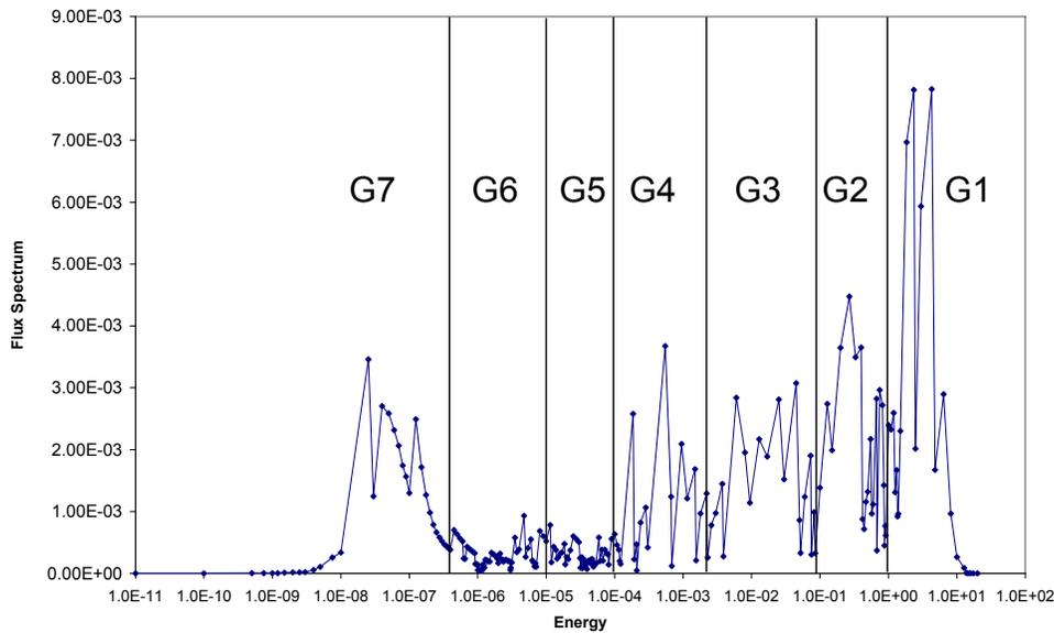
Figure 3: The flux spectrum for the fuel plate unit cell with the selected group structure indicated by the vertical divisions on the plot.
