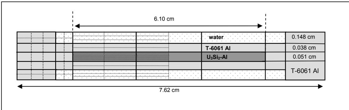
Figure 4: Illustration of the fine spatial meshing (on the left half of the figure) coarse spatial meshing (on the right half of the figure) and the as used in PENTRAN
