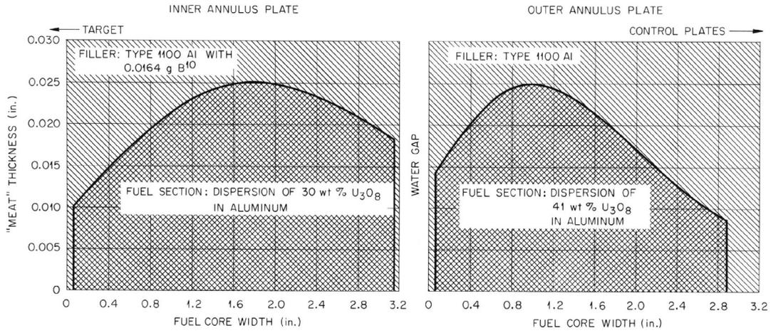
**Figure 2:** Schematic of axial end of inner element fuel plate
