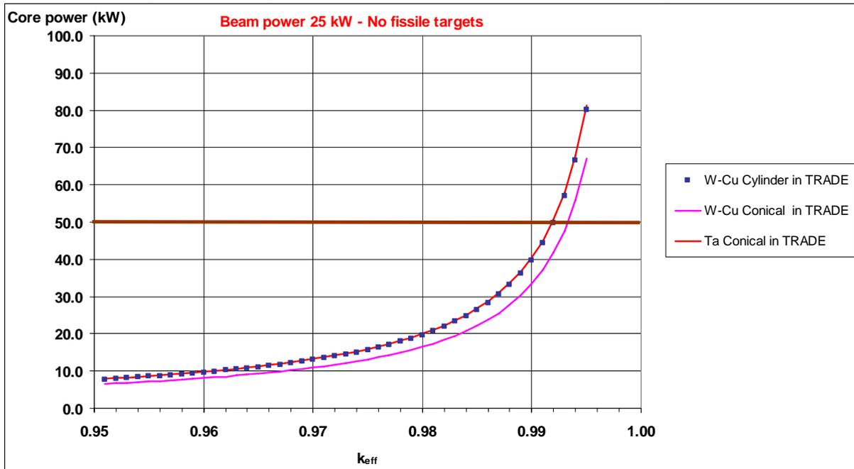
**Figure 9:** Core power vs. subcritical level for uranium targets
