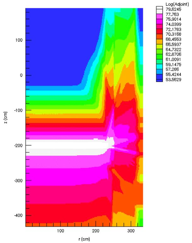
Figure 3b. Energy integrated contribution of gamma rays to the dpa/s at the core lower plate.
