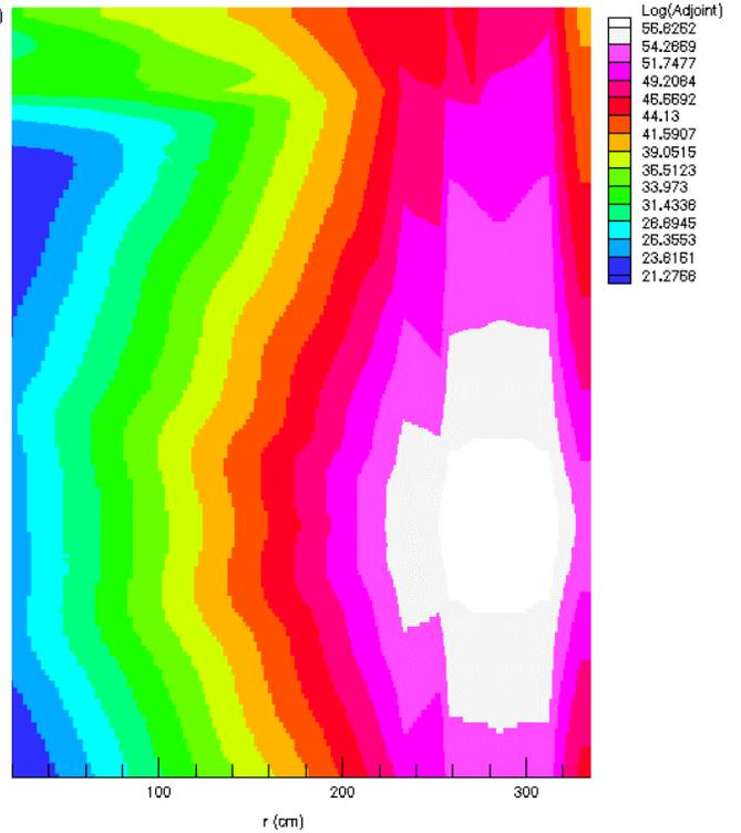
Figure 4b. Energy integrated contribution of gamma rays to the dpa/s at the jet pump assembly.
