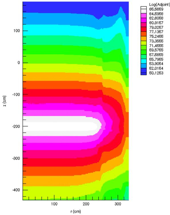
Figure 3a. Energy integrated contribution of neutrons to the dpa/s at the core lower plate.
