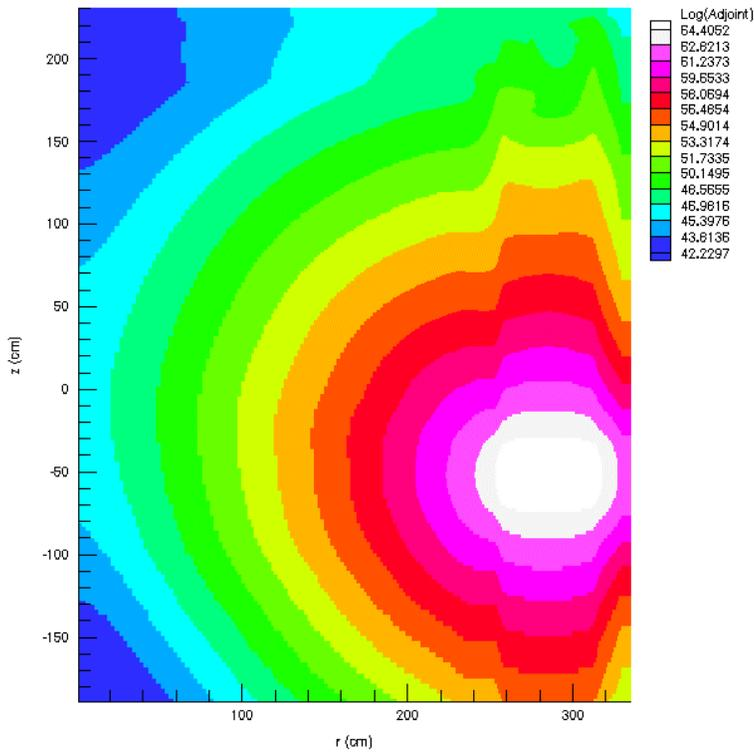
Figure 4a. Energy integrated contribution of neutrons to the dpa/s at the jet pump assembly.
