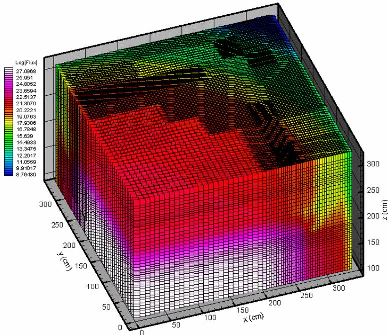
Figure 8c: Gamma flux ( $5.0 < E < 6.0$  MeV) distribution in the core top-grid and spray piping region (Model 3)
