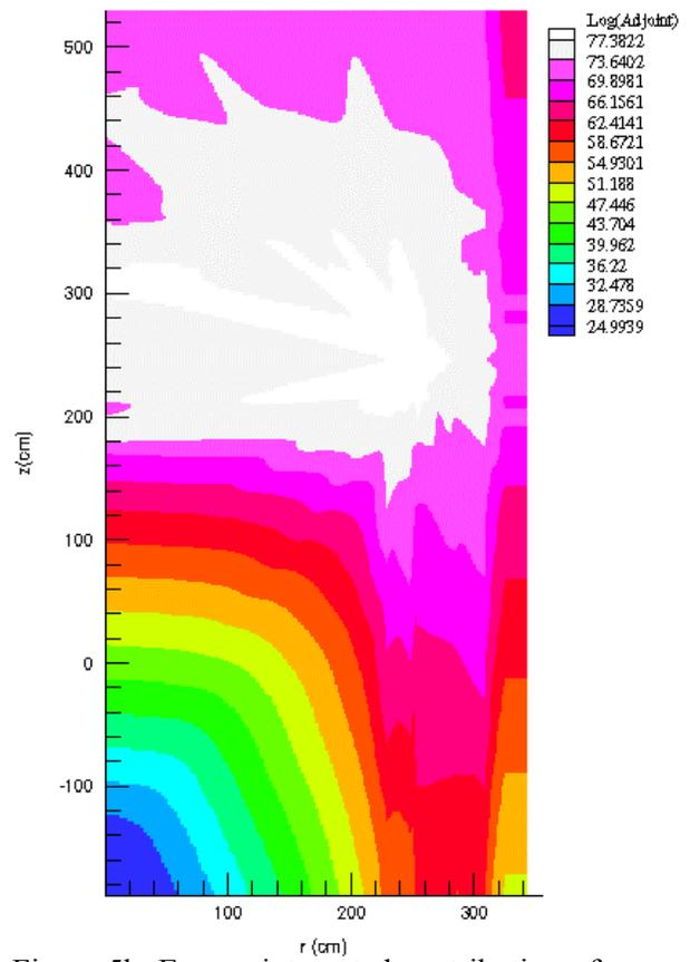
Figure 5b. Energy integrated contribution of gamma rays to the dpa/s at the core spray.
