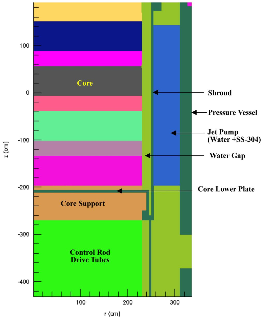
Figure 1. Model 1- Core lower plate 2-D ( $r$ - $z$ ) adjoint model
