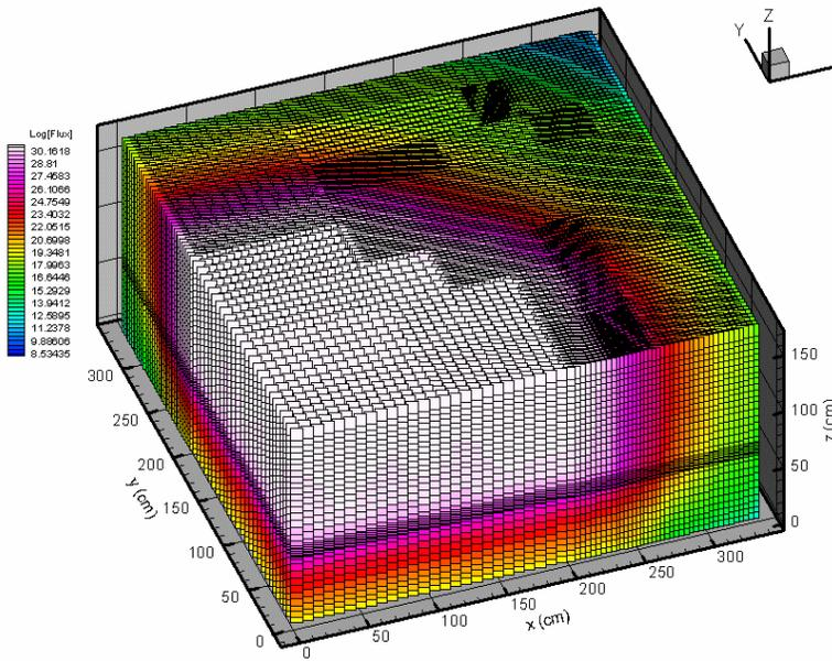
Figure 8a: Neutron integral flux ( $E > 0.1$  MeV) distribution in the core lower plate region (Model 1)
