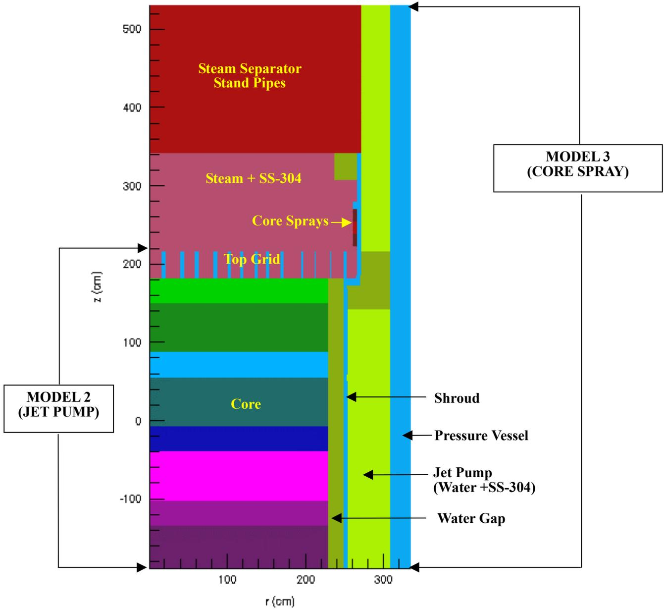
Figure 2. Models 1 and 2- Jet-pump and core spray pipes 2-D ( $r$ - $z$ ) adjoint models
