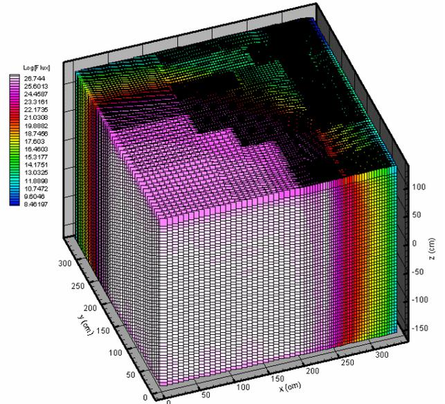
Figure 8b: Thermal neutron flux distribution ( $E < 0.257$  eV) in Model 2.
