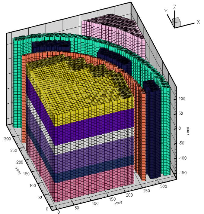
Figure 6b. Mesh and material distribution in 3-D PENTRAN model of the jet pump assembly region
