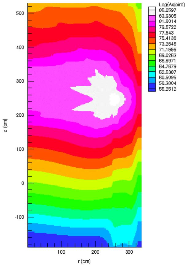
Figure 5a. Energy integrated contribution of neutrons to the dpa/s at the core spray.
