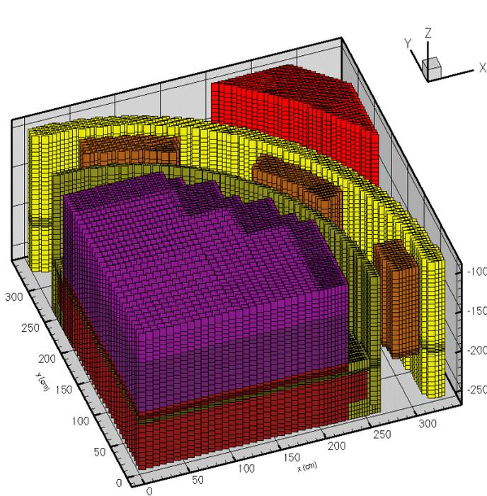
Figure 6a. Mesh and material distribution in 3-D PENTRAN model of the core lower plate region
