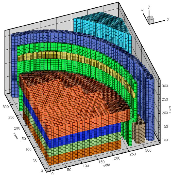
Figure 6c. Mesh and material distribution in 3-D PENTRAN model of the core spray piping region.
